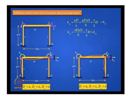
So, here only theta one only D one is there and, so one way to do it is you remove that restraint then you deliberately give an external moment that moment you need to apply to make the joint rotate by a unit angle is K 1 and the reaction that develops at the other artificially fixed end at B is K 2 1 and the reaction that is developed in the direction of the coordinate you identified in the translation degree of freedom is called K 3 1.
