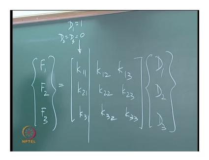
So, shall we call it D 1, D 1 should be 1, D 2 should be 0. Can you sketch the deflected shape of such a frame? Do it. Sketch the deflected shape we are trying to find the first column, so to fill this column we need to put right draw a sketch, what will it look like? it should look like this, right? It should look like this
