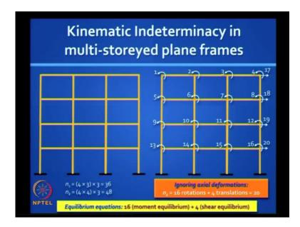
Normally, our buildings do not look that funny, you do not have inclined column you do not have inclined beam you have frames which are called reticulated frames made up of rectangles where your life is made easier and if you say axial deformations are negligible, then you have only one rotational dig unknown at every joint and one sway degree in every floor, right.
