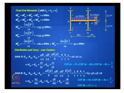
Well, first we calculate the fixed end moments for the column elements they are no fixed end moments because there is no lateral element on those columns. For the beam
