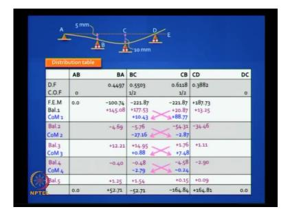
So, this is the distribution table, as you can see from the number of lines I have drawn you do not get it in one cycle. So, how do we do this? first you write down the element numbers, write down the distribution factors please note at any joint the sum of all the distribution factors should add up to one then you write down the carry over factors and you write down the fixed end moments in this case the fixed end moments are caused by the support settlements right?
