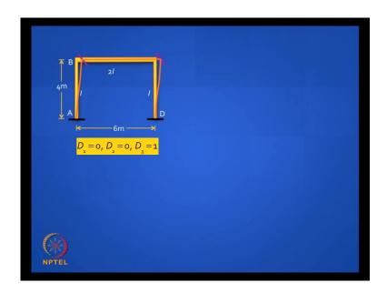
It is like a rigid beam this is how it is going to move? Point of contra flexure will be in the mid height of every column, so what will it look like? Can you calculate? can you calculate K 1 3 and K 2 3, it likes settlement of supports it likes settlement of supports it is a chord rotation, so what is the moment that you get? K 1 2 and K 2 3.
