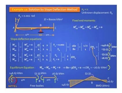
How do we solve this problem?. So, let us solve them by slope deflection method. Let us take the first problem; write down the slope deflection equations for spans AB and BC; Very simple; these equations, the first set of equations and blindly apply them.
