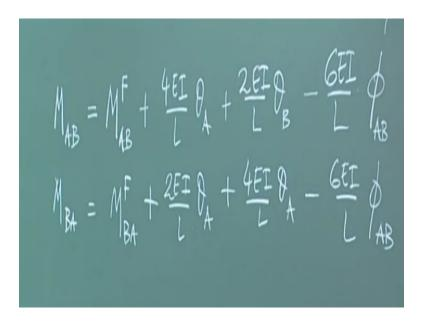
$M_{AB}$  is equal to  $MF_{AB}$  plus 4 EI by L theta<sub>A</sub>. Of course, EI by L belongs to the element AB plus 2 EI by L theta<sub>B</sub> minus 6 EI by L into phi, which is phi<sub>AB</sub>. Incidentally, phi<sub>AB</sub> is delta<sub>B</sub> downward minus delta<sub>A</sub> divided by L and M<sub>BA</sub>.
