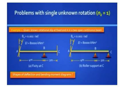
Now, let me wake you up with these problems. I have shown here two pictures of two span continuous beams. The one on the left shows you fixity at C and the one on the right shows you a roller support at C. The question at... In both these beams, you are told that somehow that fixed end at A has rotated clockwise. It is called a rotational slip by a known amount, 0.002 radius and the E I values given.
