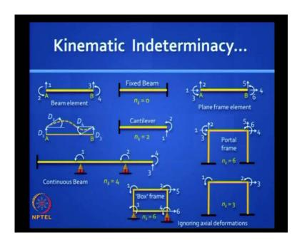
We also discussed that unlike truss elements, beam elements also have rotations in addition to translation and so you have four degrees of freedom for a beam element. The Primary Structure or the Kinematically Determinate Structure would be a one, in which all those force displacements are arrested, which is what you get in fixed beam with both ends fixed.
