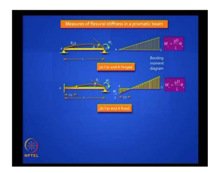
Here, the far end in this is hinged. This is a bending moment diagram and this is what we derived. Let us say that the other end A is fixed against rotation. I am not going into the proof and you should know this easily. It is going to be more difficult to rotate, if the other end is fixed; you can prove that from 3 EI by L and the stiffness goes to 4 EI by L.
