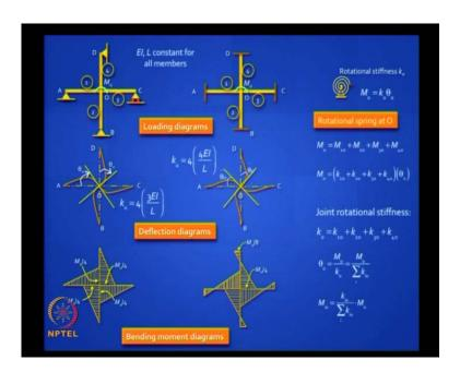
Let us demonstrate, I have got here, two frames, four members each and rigidly connected at the center at the joint O. In the first case, all the elements are simply supported at the extremities. In the second case, they are all fixed.
