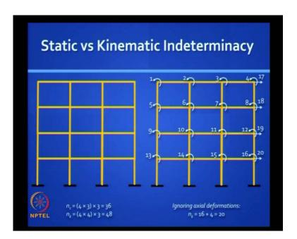
We have seen this picture earlier, here you have a four storey; three bay frame, the degree of static indeterminacy is 36 and kinematic is 48, but if you make the assumption, which we normally do is that axial deformations are negligible, then the translational degrees of freedom reduces to four.1 sway degree in each floor and that means, entire beam in any floor will move like a rigid body, horizontally.
