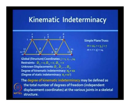
Again just to recall, kinematic indeterminacy refers to the degrees of freedom. You need to look only at the joints. In this truss for example, you have seven joints and it is a
