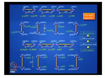
Add the two end moments in the beam divide by the span of the beam, so that is right you guys are good you can do this, so what do you get? 5 into 2 divide by 3 is 3.33 you got all the shear forces in the in the top 25 into 2 divided by 3 you got all those shear force no, no please note the shear forces are going to change because the span of the
