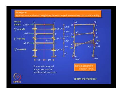
Okay, now take a look at this frame. If you assume hinges at the middle of all the beams which is 100 percent accurate and you assume hinges, internal hinges at the mid heights of all the columns which is not accurate which is a big assumption you actually introduce nine moment release locations right?
