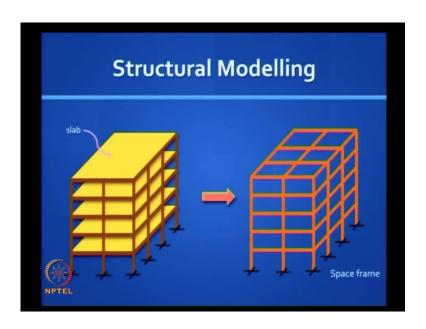
Let us look at the structure properly. So, I have shown here the picture of a building it is a it is pretty complicated you have slabs, you have columns, you have beams, and you have foundations. So for our convenience, we try to separate out the slabs which we deal with independently and separately and we transfer the loads of that slab to the to the frames, so you end-up dealing with the analysis of a space frame.
