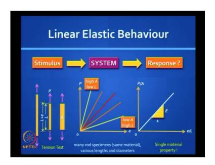
Linear Elastic Behavior and I have asked this question earlier, let us say you do a tension test on a material you can do this in the laboratory you apply a tension P and the bar elongates by E you plot P verses E you get a straight line, if you have linear elastic behavior when you unload it will retrace a path and go back to the origin but, you will find that this line will depend on the type of specimen that you tests.
