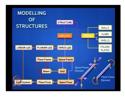
The space frame is made up of elements, which are or the structures are whole is made up of elements which are skeletal and which have also spatial elements. So, spatial elements are those elements whose plan dimensions are large, but the thickness is small for example, a slab or a plate or a shell they constitute spatial elements.
