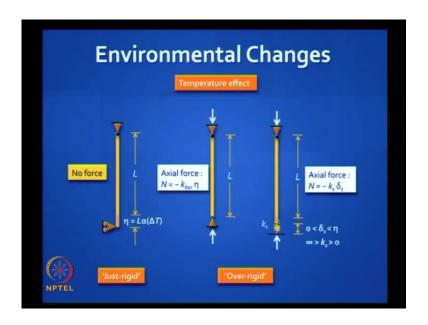
Environmental Changes. Let us take a rod like this, which is free to elongate there is no force but, let us restrain the other end either we prevent the movement fully or we put a spring there and then you have an over rigid structure you have an axial force and you can in the how much it moves depends on the stiffness of the spring.
