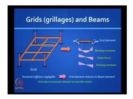
The grillages looks like this, it is all in one floor and as I mentioned the earlier the additional internal force you get is a twisting moment, which is what makes a different from one normal beam.
