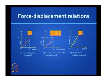
If you look carefully Force-displacement relationships P by delta is if you reduce the element to a spring to an elastic spring you use about spring stiffness right? that is called axial stiffness in this case and you will find that P by delta is the same as N by E for the simple reason that N is equal to P and E is equal to delta for a single element, so if you have different bars, you can define axial stiffness k i for the i th bar s you can prove it to be E A by L from the definition.
