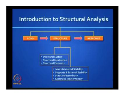
So, we have discuss this structure is really a system and the we actually deal with the mathematical model of the structure, so we reduce the complex three dimensional structure to something that we can handle so, we need to do structural idealization. We have to reduce the structure to elements and the elements are interconnected with joints and there is something called internal stability of the structure.
