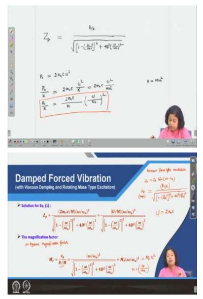
So, as I said previously, we have seen capital ZP is equal to P0 by k times 1 minus omega by omega n whole square, entire thing is under whole square plus 4 D squared times omega by omega in whole square. Now, in case of rotating mass type excitation P0 is equal to 2 times m r times e times omega square. So, what we can write from here?
