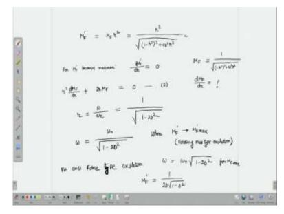
So, I would like to just write the steps here, so that one can follow and derive it. So, in case of rotating mass type excitation, magnification factor can be written as MF times r square. MF is the magnification factor for constant force type excitation. Or I can write it also as r square times 1 minus r square 1 minus r square whole square plus 4 D square r square.
