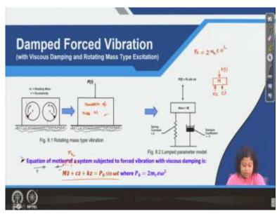
So, let us take this example. What is going on here? Actually, the excitation is created by rotating two masses one mass here, its mass is mr and this one also having the same mass mr. These two are allowed to rotate in two opposite directions. So, one is rotating, you can see this one is rotating counter clockwise direction and this one is rotating clockwise direction with an eccentricity e to the center. So, as a consequence, what is happened?
