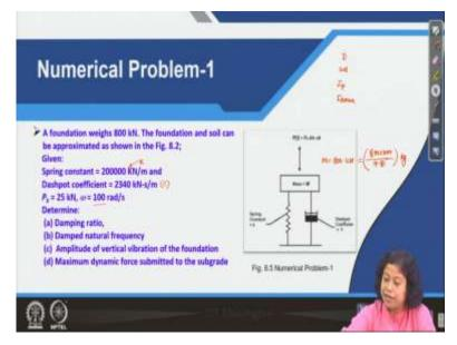
So, with this we can try to solve one numerical problem which is given here. A simple problem. So, a foundation, this one has weight 800 kilo newton that means your capital M is 800 kilo newton which we can write also as 800 into 1000 divided by 9.81 in newton by g. So, basically, it will be in kg and that is the unit for mass. Next, what is stated?
