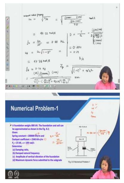
In this case, mass is given, k is given, so, we can find out first the natural frequency, undamped natural frequency. That is square root of k by capital n. Now, square root of capital, so, k is 200000. This is in kilo newton per meter. So, I can multiply it by thousand and change the unit in newton per meter then. So, now it is in newton per meter and M is 800 times thousand divided by 9.81. So, let us see, how much is the natural frequency?
