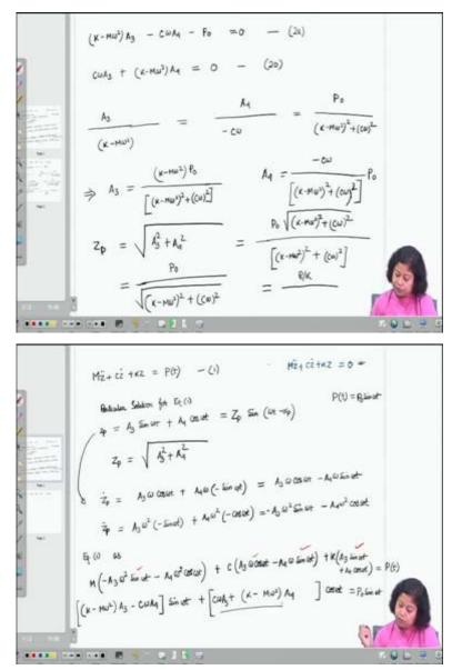
So, first one which we can write is K minus M omega square times A3 minus C omega A4 is equal to P0 or I can take P0 also on the left hand side in such case I will write it as minus P0 is equal to 0, give it a name 2a. Next equation, so first equation is formed, now next equation will be from this one.
