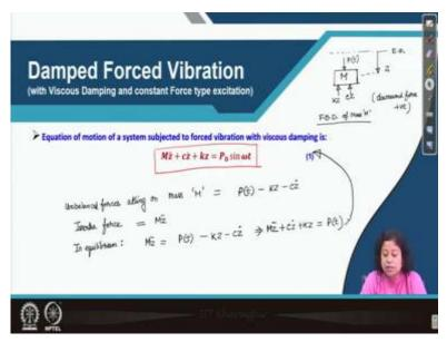
So, in this case first we will see the equation of motion. Here you can see the equation of motion the question you may think or ask that how this equation is coming. So, let us first draw the free body diagram for the mass M, mass M means which represents the foundation so it is resting on the soil.
