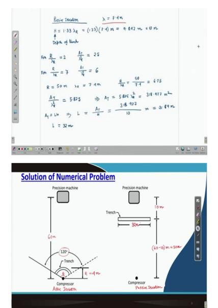
So, for passive isolation we have to follow a few steps to for the design. So, let us see what are the steps for passive isolation? So, first we will find out the depth of the trench that means H. We have already gone through the rules, so what it is said H should be equal to 1.33 times of lambda R. What is lambda R? It is the wavelength of the Rayleigh wave. So, already we have calculated lambda R, which is equal to 7.4 meter approximately.
