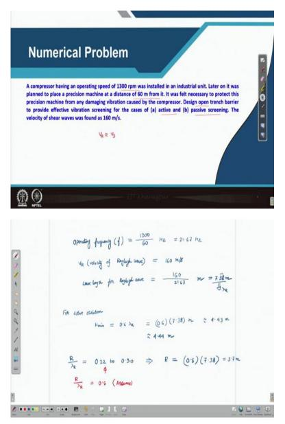
So, let us take one numerical problem. So, in this problem what is asked - A compressor having an operating speed 1300 rpm was installed in an industrial unit. Later on, it was
