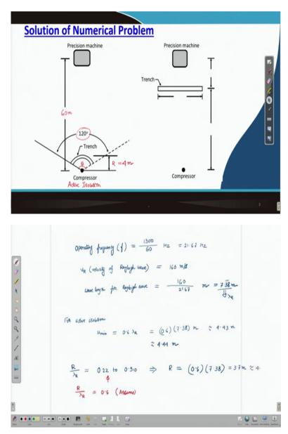
So, this is the case for active isolation. I made a spelling mistake, let me correct it. So, this is the case of active isolation. So, here you can see this is the source of vibration, which is trying to isolate. So, this, how it is doing by excavating a trench. Now, in this case what I need to mention, you can see already said the distance between compressor and this machine, it is 60 meter, so I can write here this is 60 meter which is given also.
