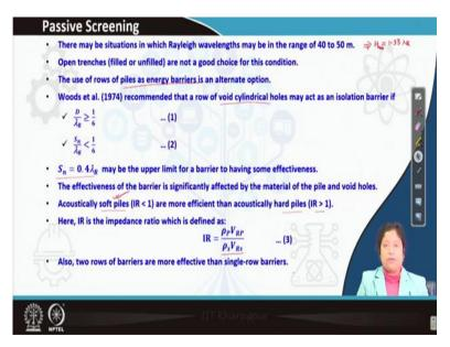
Now, we can go to the next topic, actually this is important, we have seen how to calculate the H and L, that means depth and, how to calculate depth and length of the circular trench. Now, they are sometime what is happen, the wavelength of the Rayleigh wave may be found in the range of 40 to 50 meter, so if the wavelength is 40 to 30 meter, then you can imagine what is the H value, it is minimum 1, I can write minimum 1.33 times lambda R.
