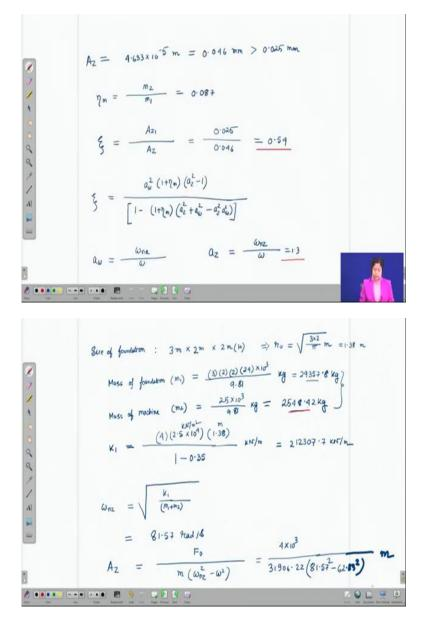
So, xi means, sorry, xi means 0.54 which is equal to a omega square times 1 plus 0.087, this is eta m times 1.3 square minus 1, 1.3 square means Az square divided by 1 minus 1 plus eta m which is 1.087 times Az square, Az square means 1.3 square plus a omega square minus 1.3 square times a omega square. This is the expression now using the value of xi and Az and also eta m. So, with this now we can find out a omega square.
