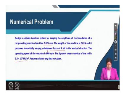
So, this is the problem which we are interested to solve today. Design a suitable isolation system for keeping the amplitude of the foundation of a reciprocating machine less than 0.025 millimeter. That means, permissible amplitude of vibration of the foundation is already provided. The weight of the machine is 25 kilo Newton and it produces sinusoidally varying unbalanced force of 4 kilo Newton in the vertical direction.
