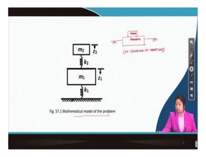
So, if I go to the next page, here you can see, basically this is the mathematical model of the problem with the vibration isolator. Actually, how machine is resting, this is the machine, it is resting on the foundation. Now, there is a possibility of excessive settlement, so this is machine, this is foundation, so no isolation for this case, isolation of vibration.
