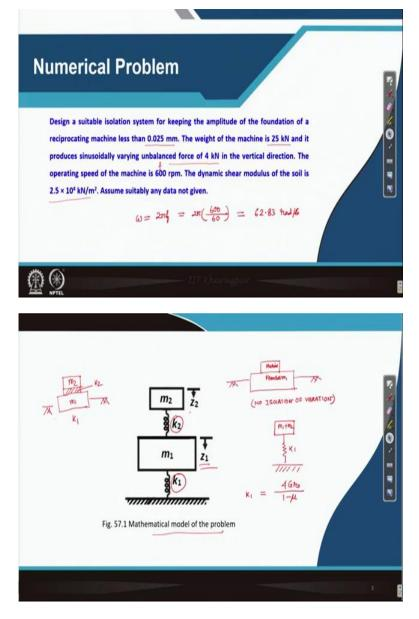
So, let us go to the white bard. We can assume data for the size of the foundation because it is not given here. So, let us take size of foundation that is 2 meter by 3 meter by 2 meter. So, this, I can write it 3 meter by 2 meter that looks, 3 meter by 2 meter by 2 meter. So, last one is height. That means what is the volume that we can calculate from this information?
