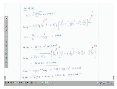
So, for pile cap first we need to find out the equivalent radius r0. So, r0 for pile cap is let us see what is the area for pile cap area is 3.4 meter by 3.4 meter. So, equivalent radius is equal to square root of 3.4 square divided by pi and unit is in meters so, we are getting r0 for pile cap is equal to 1.918 in meter.
