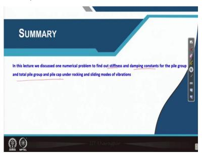
So, then we can come to the summary of today's class as you know, we have discussed the numerical problem to find out the stiffness and damping constants for the pile group and total pile group and pile cap under rocking and sliding modes of vibrations.
