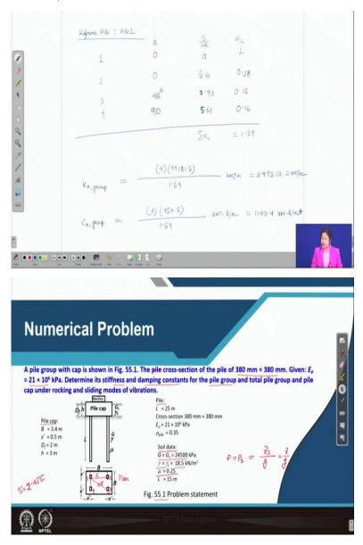
So, I am going to the new page here reference pile let us take a reference pile is pile 1 pile number 1. So, whatever we will calculate that is to find out alpha L that is with reference to pile number 1. Now, for what are the different points for which we need to find out alpha L for pile 1, 2, 3 and 4 and it depends upon beta it depends upon SS divided by 2R it means the value of alpha L.
