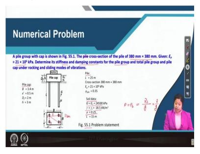
For that we need to also find out S divided by 2R this ratio from the given problem, so, here what we can see you can see here, what is the spacing between two piles, since it is a square shape pile cap. So, these things center to center distance is so, these we will measure the distance and that is S and already the value for R is known. So, from that we can calculate the S divided by 2R value. So, this is for let us give some number for the 44 different piles.
