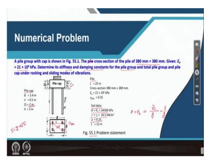
So, from these now, from with these information now, we will find out Kx for pile cap and for that we can use the equation Gs times Df times S x1 or S bar x1 and for Cx cap this is equal to Df times r0 times S bar x2 times square root of Gs times rho s, so, Gs and rho s are shear modulus dynamic shear modulus and rho s is density of the backfill soil respectively. So, and Df refer the figure here Df is said 2 meter.
