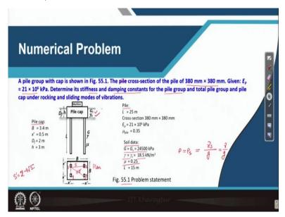
So, for that once again I am going back to this figure. So, here what we can see pile cap is embedded in the soil or I can say after placing pile cap, backfilling is done by the soil and you can see the gamma S and Gs value for the backfill soil.
