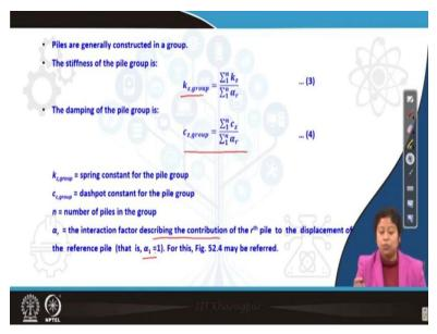
Now, piles are generally constructed in a group. So, when pile is in a group, then we need to find out the stiffness of the pile group. How we will do that? We know the stiffness of individual pile. So, if we will sum it and the sum will be divided by interaction factor alpha r, then summation of alpha r; then we will get the Kz for pile group. Similarly, the damping of the pile group is Cz group and that can be calculated using equation 4 here.
