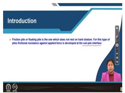
So, in last class we have discussed the end bearing pile subjected to vertical vibration. Now, the second type of pile is friction pile or floating pile. So, that is the one which does not rest on the hard stratum. So, basically for this type of pile it is penetrates; it is, it penetrates through the good quality of soil stratum And for these type of piles, frictional resistance against the applied force is developed at the soil pile interface.
