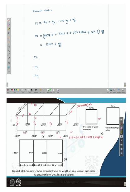
So, for horizontal vibration we need to do a little bit calculation. So, that I am showing. So, we know that we need to find out, that means, total mass acting on that frame is equal to mmi
