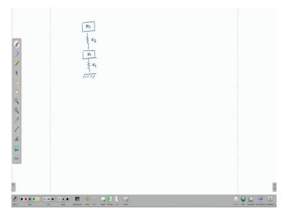
So, in amplitude method we already learned that the frame foundation will be represented by a 2 degree of freedom system, this is mass m2, this is mass m1, k2 and this is k1. So, here we need to know what is how to calculate k1, k2, m1, m2, etcetera. So, let us take the frame 1.
