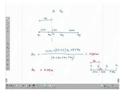
Then what we need to do? This is the original position of the deck. So, this is m1, this is m2 this is m3 and this is m4. So, this distance is 2.5 meter, this distance is 3.2 meter and this distance is 4 meter.
