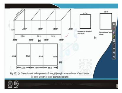
So, in this numerical problem here you can see the diagram also, we are interested to solve this frame foundation. This frame foundation is for a turbo generator. So, what we have done last class, we have calculated the average natural frequency of the system when it is subjected to vertical vibration.
