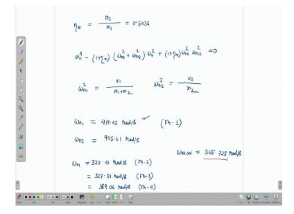
So, here what you can note is that I am just going back to previous pages. So, here if you see earlier when we solve the problem using resonance method we get omega n z average is equal to 369.67 radian per second. Right now when we solve the same problem using amplitude method what we get is 365.725. That means, this time we are getting slightly lower value.
