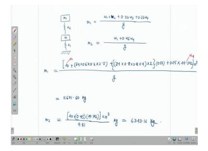
So, for this frame, for any frame actually, m1 is equal to w1 plus w2 plus 0.33 w3 plus 0.25 into w4 and this is divided by g. Likewise we can calculate m2, which is equal to w1 plus 0.45 w4 divided by g. Now, the question how we will calculate w1, w2, w3 and w4? So, w1 we already, we can get the information of w1, from here you can see w1 is 40 kilo Newton which is the weight on the cross beam of each frame. Now, what is w2? So, w2 is basically the weight of, the self-weight of this beam.
