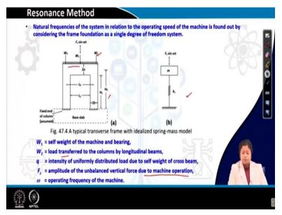
So, now we will study how to do the two-dimensional analysis. Already I told there are three methods; first one resonance method, second one amplitude method, and the third one is the combined method proposed by major.
