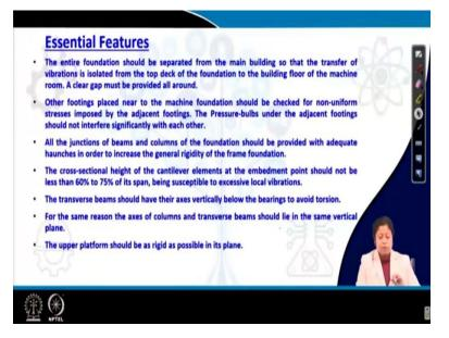
But, before that we will discuss few essential features. So, the first feature is the entire foundation should be separated from the beam building, so that the transfer of the vibrations is isolated from the top deck of the foundation to the building floor of the machine or machine room.
