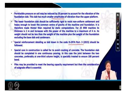
Now, the permissible pressure on soil may be reduced by 20% percent to account for the vibration of the foundation slab. This slab has much smaller amplitude of vibration than the upper platform. The lower foundation slab should be sufficiently rigid to resist non-uniform settlement and heavy enough to the lower, sorry and heavy enough to lower the common center of gravity of the machine and foundation.
