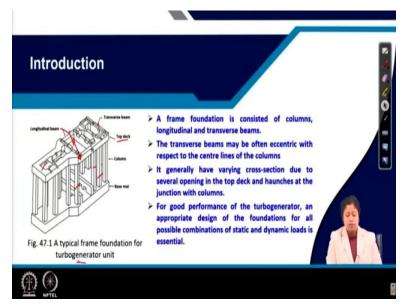
Now, in this figure, you can see a typical frame foundation which can be used for turbogenerator you need. So, what are the different components that we need to see here? You can see base mat which supports these columns, a series of columns you can see here; this is also columns, this is also columns. Now, the columns supports top deck, and it will be better to say columns supports transverse and longitudinal beams on which these top deck is resting.
