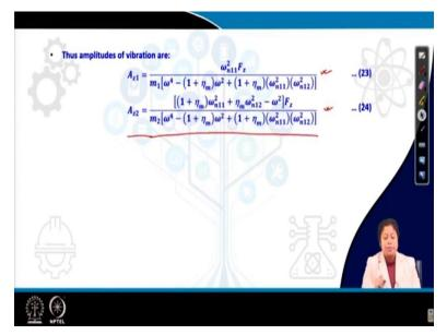
So, amplitudes of vibration Az1 can be expressed by this equation. Likewise, Az2 which is the amplitudes of vibration for the mass m2, that can be determined by using the second equation. So, equation 23 and 24 provide the amplitudes of vibration Az1 and Az2.
