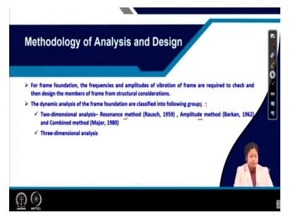
Now, considering all these four load combinations, our next target is to learn the methodology of analysis and design of machine foundation. So, for frame foundation, the frequencies and amplitudes of vibration of frame are required to check, and then the design the members of the frame from structural considerations.
