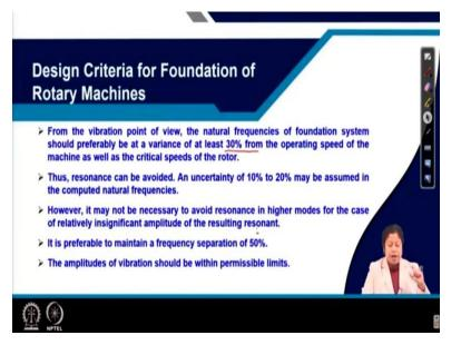
Now, let us see the design criteria for foundation of rotary machines. From the vibration point of view, the natural frequencies of foundation system should preferably be at a variance of at least 30 percent from the operating speed of the machines as well as the critical speeds of the rotor.
