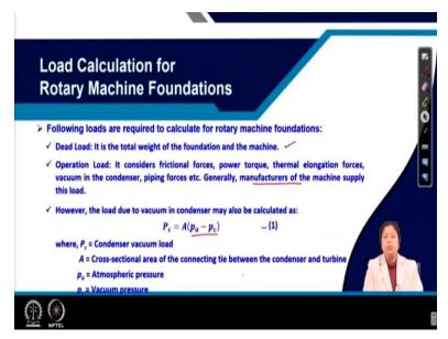
Now, how do we do the load calculation? For load calculation for rotary machine foundations, we need to consider four combinations of loading. So, before knowing all these four combinations of loading, first we need to know what are the different loads. First one dead load; it is the total weight of the foundation and the machine together.
