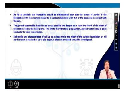
As far as possible, the foundation should be dimensioned such that the center of gravity of the foundation with the machine should be in the vertical alignment with that of the base area in contact to the soil. The groundwater table should be as low as possible and deeper at least one-fourth of the width of the foundation below the base plane.
