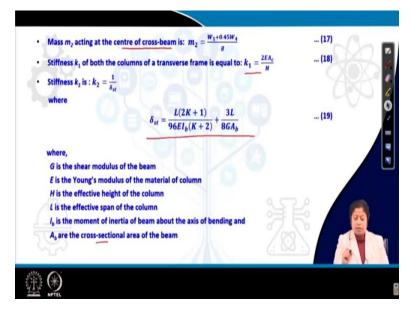
Now, next is to calculate the mass m2. So, mass m2 acting at the center of cross-beam is W1 plus 0.45 times W4 divided by g. Next, we need to calculate stiffness K1. K1 is the stiffness of both the columns of a transverse frame; so, there are two columns. So, for both the columns, this stiffness K1 can be calculated using equation 18. That can be calculated using the expression, 1 divided by delta st, where delta st is this expression shown in equation 19.
