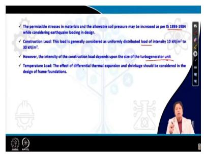
Now, the in presence of seismic load what is happening? The permissible stresses in materials and the allowable soil pressure may be increased as recommended in IS 1893, while considering earthquake loading in design; so, we need to take care of this point as well.
