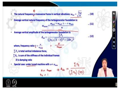
So, if we are able to calculate the mass or total weight W, either total mass m or total weight W; from that we can calculate the natural frequency of a transverse frame subjected to vertical vibration using this equation. Already, we know how to calculate W.
