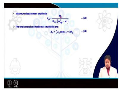
So, the maximum displacement of course in this case it is rotation is how much My divided by M mo times this one. This is the amplitude. So, basically here it will be M 0y. Let me check the figure once again, yes M 0y we have to consider here. And from this we can calculate that total vertical and horizontal amplitudes as shown in equation 14.
