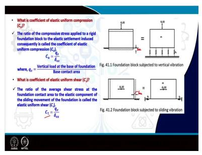
The first question is what is coefficient of elastic uniform compression? Let us see its definition. It is the ratio of the compressive strength applied to a rigid foundation block to that elastic settlement, which is induced consequently in the foundation is called the coefficient of elastic uniform compression. So, here you can see Cu is equal to qz divided by delta ez.
