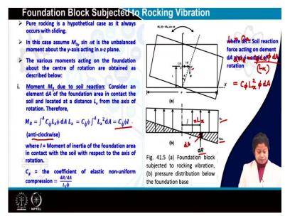
Now, let us see the third mode of vibration, which is rocking vibration that means, in this case, the foundation block is subjected to rocking vibration. So, in figure a, we can see a foundation is subjective to rocking vibration and consequently it is tilted by an amount pi. Now, here what you can see, because of this tilting. it is CG. Originally, CG was located at O, which is shifted to O dashed now. So, the distance between O and O dashed is n times pi,
