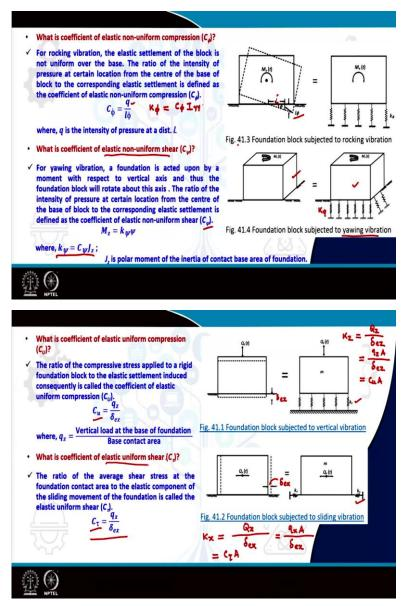
So, the next question is what is coefficient of elastic non-uniform compression? So, basically what is happening when a foundation is subjected to rocking vibration? It is tilted on either
