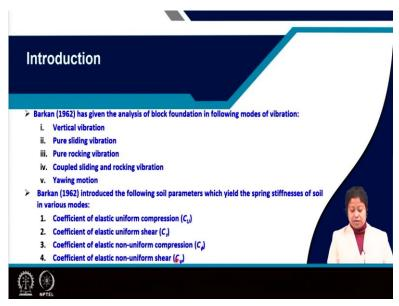
So, the method which we are discussing today is proposed by Barkan in 1962. What he said, he given the analysis of block foundation in the following modes of vibrations, what are those modes? Vertical vibration, pure sliding vibration, then pure rocking vibration, coupled sliding and rocking vibration and yawing motion. Now, Barkan also introduced a few soil
