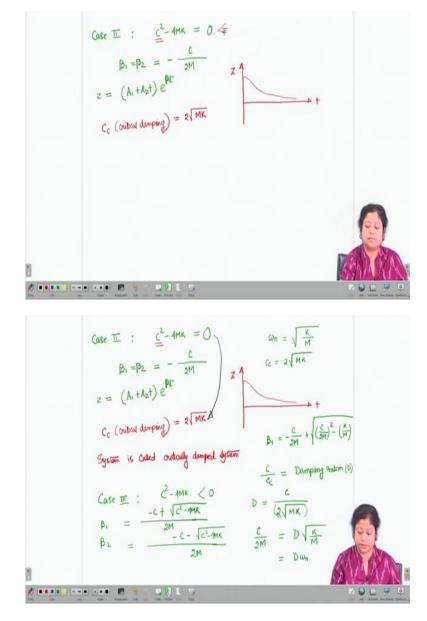
We will get M times Z double dot means A times beta square e to the power beta t plus C Z dot which is nothing but A times beta times e to the power beta t plus K Z that means K times A times e to the power beta t which is equal to 0. Now, it can be rewritten as M beta square plus C times beta plus K times, plus K whole thing can be multiplied by A times e to the power beta t and that should be equal to 0.
