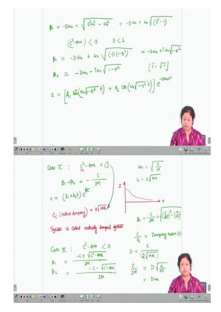
Then beta 1 is equal to, sorry beta 1 is equal to minus D omega n plus square root of D square omega n square minus omega n square or I can write it as D times omega n plus I can take omega n outside the square root and it will be D square minus 1. Now, under underdamped condition when C square minus 4 M K this is less than 0 that means negative that time obviously D is less than 1.
