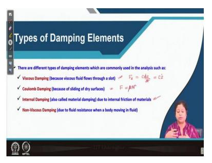
Now, let us see what are the different types of damping elements. There are different types of damping elements which are commonly used in the analysis such as, viscous damping it is present because of the flow of viscous fluid through a slot. Next is coulomb damping which is present because of sliding of dry surfaces on each other? Internal damping is also called as material damping which is due to internal friction of the materials.
