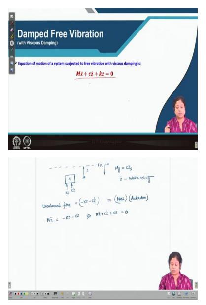
So, in this case we can derive the equation of motion of this system which is subjected to free vibration and connect it to viscous damping, let us see. So, first thing what we need to do is to draw the free body diagram of the mass M. So, this is our mass M, we have already seen that when external forces are not present, we can write M g is equal to K times of Z S, where Z S is the static displacement of the mass M under the action of the load M g.
