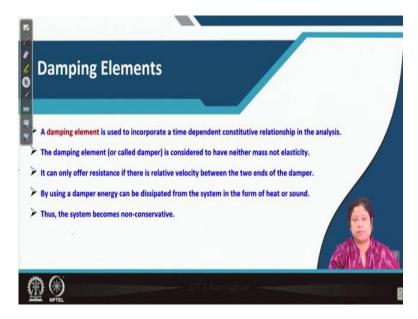
So, our today's topic is damping, so first we will see what is damping element. So, a damping element is generally used to incorporate a time dependent constitutive relationship in the
