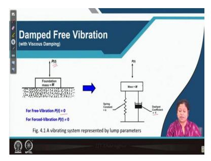
Now, let us see what will be the equation of motion for damped free vibration condition. So, in this figure we can see a foundation which is a block foundation, its mass is capital M is resting on the ground surface. Now, under free vibration condition the load P t will be equal to 0, in case of forced vibration P t will be non-zero. So, just for the sake of completeness I am just repeating what is free vibration which we have already studied.
