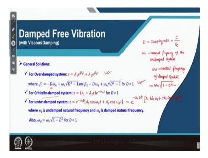
And I can show now what we have done here. So, the general solutions for the three cases which are discussed today can be summarized here, for the over damped system we get Z is equal to A 1 times e to the power beta 1 t plus A 2 times e to the power of beta 2 t. We can write beta 1 and beta 2 in terms of D which is damping ratio and the natural frequency of the undamped system which is omega n.
