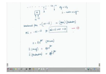
Now, we are interested to find out the general solution for this equation. For this purpose what do we do? We will assume that Z, it is better to write it as small z, z is equal to A times e to the power beta t, this is solution which we assume right now and this kind of trial solution we can take for differential, homogeneous differential equation having form this.
