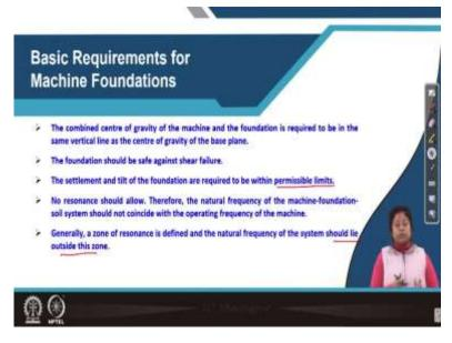
So, now, let us see what are the basic requirements of machine foundations. The first requirement is the combined center of gravity of the machine and the foundation is required to be in the same vertical line as the cg of the base plane. So, both the CG should be in the same vertical line. Second criteria is requirement is the foundation should be safe against shear failure the settlement and tilt of the foundation are required to be within permissible limits.
