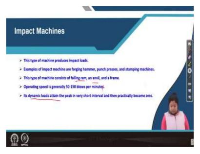
Now, the second type of machines which we encounter is impact machines, this type of machine produces impact loads, what is the characteristics of impact loads? These type of let us see the characteristic first basically these dynamic loads attain the peak in very short time interval and then practically becomes zero.
