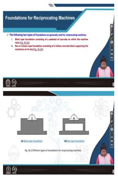
Now, let us see what type of foundations can be provided for reciprocating machines. There are 2 types of foundations that are generally used for reciprocating machines one is you can see blocked type foundation consisting of a pedestal of concrete on which the machine will
