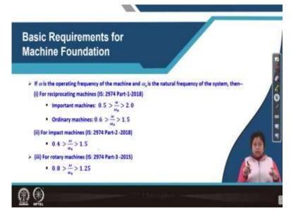
So, let us see what is the zone of resonance for different types of machine foundations. So, if omega is the operating frequency of the machine and omega m is the natural frequency of the machine foundation soil system then for reciprocating machine what is the resonance zone? If it is important machine then resonance zone is 0.5 to 2 that means, the ratio of omega by omega n either should be less than 0.5 or should be more than 2.
