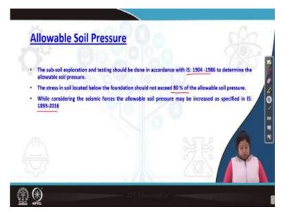
Now, the next important parameter is soil pressure or allowable soil pressure. The subsoil exploration and testing generally is essential in accordance with IAS 1904 published in 1986 to determine the allowable soil pressure, the stress in soil located below the foundation should not exceed 80 percent of the allowable soil pressure. Now, while considering the seismic forces the allowable soil pressure may be increased as specified in IS 1893 published in 2016.
