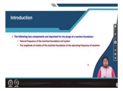
So, now, then what are the components for the machine foundations are required to check that there are 2 components which are important when we are designing machine foundation these are natural frequency of the machine foundation soil system. So, we will consider together the machine foundation and the soil and its natural frequency is a subject of our concern. Second important component is the amplitude of motion at the operating frequency of machine.
