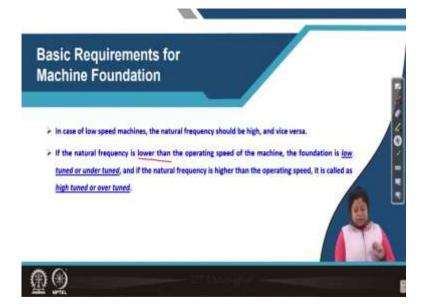
Now, in case of low speed machines the natural frequency should be high and for high speed machine the natural frequency should be low. This is a simple guideline when we are designing and analyzing the machine foundation. Now, when the natural frequency of the machine foundation soil system is lower than the operating frequency of the machine we call the foundation is low tuned or under tuned.
