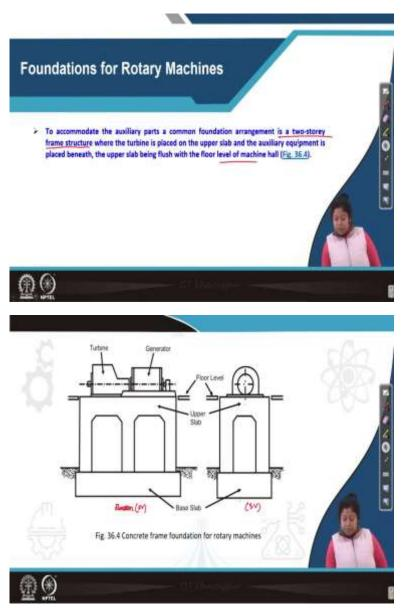
Now, what is total unbalanced force in vertical direction that is, so, what type of foundations we will choose for these types of rotary machines. To accommodate the auxiliary parts which I have presented in previous slide what we used to do a common foundation arrangement is a 2 storey frame structure, where the turbine is placed on the upper slab and the auxiliary equipment is placed beneath, the upper slab being flush with the floor level of the machine hall.
