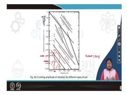
Generally, the amplitude of motion at operating frequencies must be within the permissible limit. So, the permissible amplitude should not exceed the limiting amplitude of the machine which is generally provided by the manufacturer. The vibrations neither be annoying to other persons working in the factory nor be damaging to other precision machines. Now, we can see a chart which is provided by Richard to give various limits of frequency and amplitude for different purposes.
