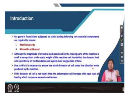
So, first we need to understand what is the difference? Where is the difference? Or what is the difference when a foundation is subjected to static loading and when it is subjected to dynamic loading. So, for general foundation, when it is subjected to static loading, we need to ensure 2 essential components what are those components first are bearing capacity and another important component is allowable settlement.
