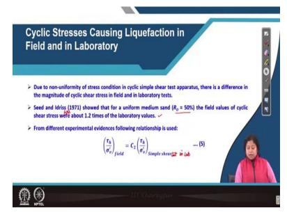
Now, we will discuss the cyclic stresses causing liquefaction in field and in laboratory. What is happened when we are doing (sim) cyclic simple shear test in the lab, because of some constraint in the apparatus non uniformity of stress condition in cyclic simple shear test apparatus is noted and consequently, there is a difference in the magnitude of cyclic shear stress in field and in lab test.
