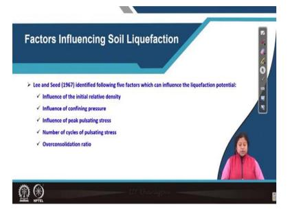
Let us see what are the different factors that influence soil liquefaction Lee and Seed 1967 identified five factors which can influence the liquefaction potential of soil. First one is initial relative density, then confining pressure, then peak pulsating stress, number of cycles of pulsating stress and over consolidation ratio of soil.
