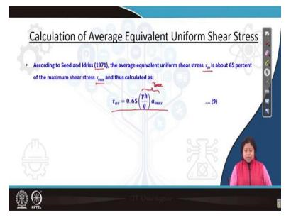
Now, according to Seed and Idriss, 1971 the average equivalent uniform shear stress which is tau average is about 65 percent of the maximum shear stress tau max and that can be calculated by using this equation. So, here if you see basically, this is tau max and tau max is multiplied by 0.65 to consider the average equivalent uniform shear stress.
