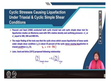
Now, we will see cyclic stresses causing liquefaction under triaxial loading condition and under cyclic simple shear condition. So, Peacock and Seed in 1968 conducted both cyclic triaxial test and cyclic simple shear test for liquefaction studies for a particular sand and it is they have done the experiment at a particular relative density and confined three different confining pressures, which are mentioned here.
