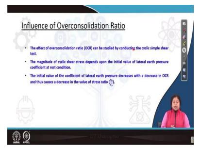
Let us see that influence of overconsolidation ratio. What is over consolidation ratio? Generally, it is the ratio of the pre consolidation stress to the current vertical effective stress in the soil. So, the effect of overconsolidation ratio can be studied by conducting cyclic simple shear test not by dynamic triaxial test.
