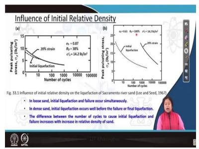
So, first we will see the influence of initial relative density here. So, in Figure a is for loose sand where Lee and Seed has taken a Sacramento river sand and the characteristics of this sand in loose state which was considered at the time of experiment was given you can see here e0 is the initial void ratio Rd is the relative density and sigma 3 dash is the effective confining pressure.
