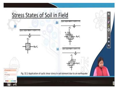
So, what is the stress states of soil in the field when there is no earthquake and when there is earthquake. So, when there is no earthquake, we can see the figure a what is happened? Vertical effective stress is acting on the soil element. Also, since the soil is at rest condition, so, lateral stress having magnitude k0 times sigma v dash acts on the soil element. Now, what is the how we can calculate sigma v dashed?
