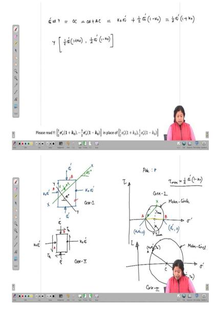
So, now if I am interested to find out the value for the stresses acting on yy plane then that I can get from this dad diagram itself shear stress you can see that is tau max. So, in this case the magnitude of tau max is already calculated. What is the magnitude of the normal stress at this point y on the Mohr circle?
