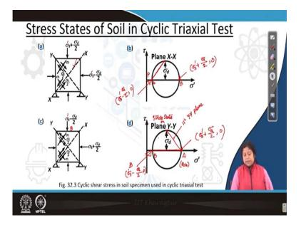
Now, in triaxial test, how we can simulate this condition? In triaxial test what we can do first we can apply the all-round pressure then we can apply axial stress additional axial stress. So, due to that reason, what we can do here is that first we will apply sigma 3 dashed which is the all-round pressure then, we will apply the axial load in such a way that the total actual stress on the horizontal plane that means total vertical actual stress becomes sigma three dashed minus sigma d.
