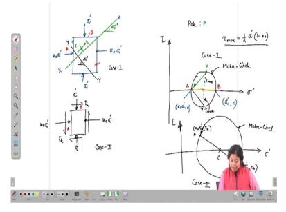
So, if this is our soil element so, on any plane we can get the state of stresses. So, we can expect one normal stress and one shear stress component. So, one component related to the normal stress the other one related to the shear stress like this we can get same thing here also, same thing here also.
