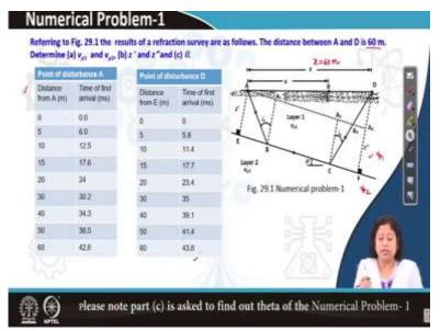
So, let us take the first problem which is shown in this figure also. So, here it is said that in figure to 29.1 the results of a refraction survey are given, the distance between A and D is 60 meter that means here x is equal to 60 meter, our objective is to determine the velocity of the P wave in layer 1 that means v p 1 here and the velocity of the P wave in layer 2 that means v p 2.
