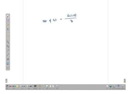
So, what I said is that slope of a 2 b is equal to sin of i c plus theta divided by v p 1, once again v p 1 is the velocity of the P wave in layer 1.
