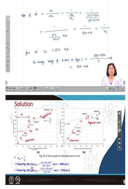
So, now slope of o a 1 dash is equal to what is the slope of this line here we can calculate delta t 2 and delta x 2, so in terms of delta t 2 and delta x 2 first I am writing the expression so delta t 2 divided by delta x 2. Now, so slope of o a 1 dash is equal to 1 divided by delta x 2 divided by delta t 2.
