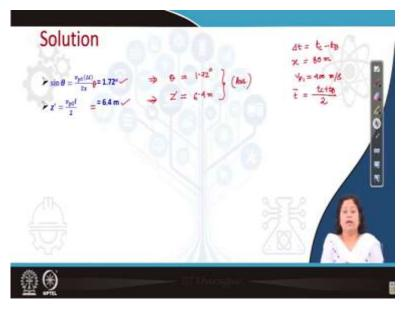
So, sin, for sin theta we can write sin theta is equal to v p 1 times delta t divided by 2x we know what is delta t, here delta t is equal to t c minus t b delta t is equal to t c minus t b so if I will write the difference of t c and t b then I will get delta t and x is already mentioned it is 80 meter so from that we can calculate the sin theta.
