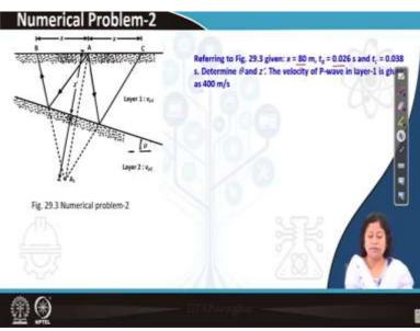
Let us take another numerical problem, in this problem we have carried out reflection survey and the distance between source and receiver is given which is 80 meter, the travel time of the P wave reflected P wave from A to C is given which is 0.038 second and the travel time of the reflected P wave from A to B is given which is t B 0.026 second, we are asked to find out theta and Z dash velocity of P wave of layer 1 is also given which is 400 meter per second. (Refer Slide Time: 30:17)
