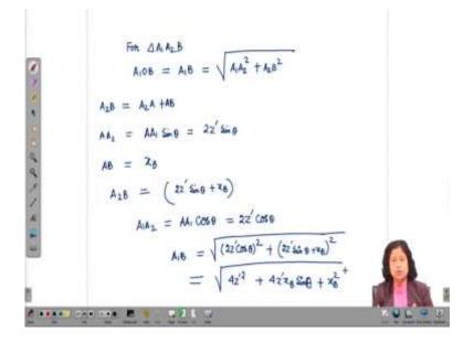
So, in previous slides, we have seen how to get the thickness of the layer one when horizontal layering is happened. Now, what will be happen when the interface of the when this layering is inclined that means, here you can see the interface of these two layer is in is one inclined plane, in that case how I will get the, how I will get that information about the layer 1 that we will now see.
