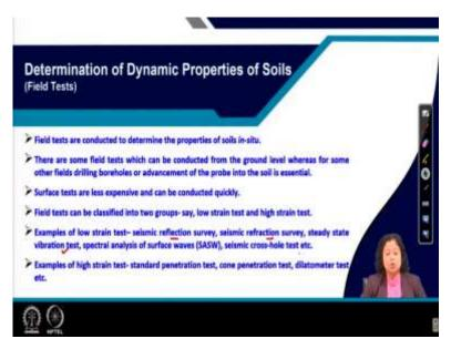
Field tests are conducted to determine the properties of soil in situ. There are some field tests which can be conducted from the ground level, whereas for some other field test drilling of boreholes or advancement of the probe into the soil is essential. Generally, the surface tests are less expensive and can be conducted quickly. The field tests can be classified into two groups, say, low strain test and high strain test.
