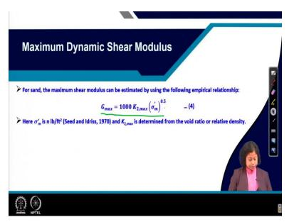
Now, for sand what will be the G max value or how do we find out the G max value. For sand generally we use we may use this equation G max is equal to 1000 times K2 max times sigma
