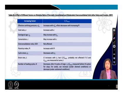
Here you can see the effect of different factors like, Effective confining pressure, Void ratio, then Over consolidation ratio, Plasticity of plasticity index of soil, Cyclic strain etcetera be on the magnitude of modulus ratio that means, G by G max. So, what we can see from this table the value of G by G max depends upon several factors which are mentioned on the left hand side column like, Effective confining stress, Void ratio.
