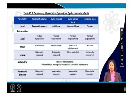
Now, in this table you can see what are the different parameters that we actually calculate or measured from different dynamic tests in the laboratory. So, first one is resonant column test. From resonant column test in terms of load actually, what we get is resonant frequency, we can also measure vertical displacement, we can, generally cannot measure the pore water pressure from resonant column test, generally we do not.
