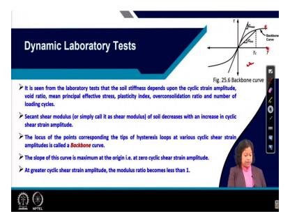
So, here is the backbone curve you can see, so, this is. Now, the slope of this backbone curve at origin that means, when shear strain is or I can say cyclic shear strain amplitude is 0 that time we get the G max, at greater cyclic shear strain amplitude that means, when now we are shifting towards this direction the modulus ratio becomes less than 1, these we have already seen in the previous slide.
