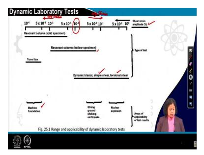
So, first we will, here we can see the range and applicability of different dynamic laboratory tests. First thing which we need to remember is the boundary between low strain test and high strain test. The boundary shear strain amplitude is 10 to the power minus 4 or I can say 10 to the power minus 2 in percentage. So, here you can see this is the boundary for low strain and high strain laboratory test. So, this side is mainly for the high strain and the site mainly for low strain.
