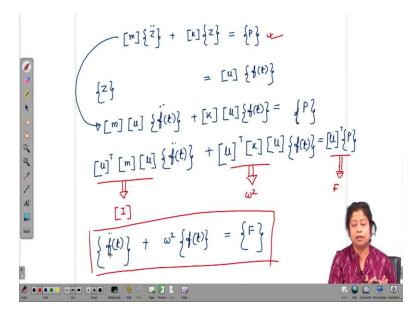
In the next step what we will do in the next step we need to just write I am writing one line we have the equation of motions that is mass matrix times z 2 dot which is acceleration vector plus k times displacement vector is equal to force that we have now, what we can do here.
