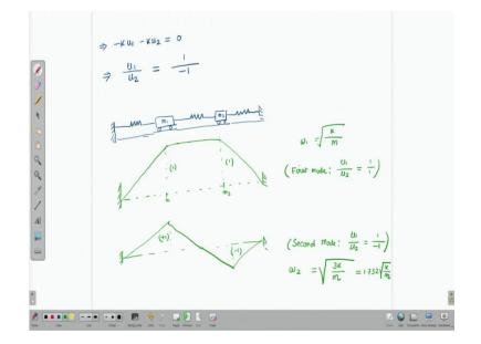
First one is for omega 1 is equal to square root of K by n, what equation 6 says I am just rewriting equation 6 in terms of omega 1 first. So, it is coming 2K minus m omega 1 square minus K minus K again 2K minus in omega 1 square. This is multiplying by U vector right hand side is a null vector. So, from these now we can get a relationship between U 1 and U 2. So, what is that relationship?
