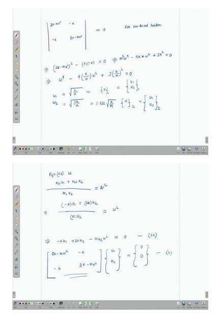
For non-trivial solution what is the procedure? The determinant of the coefficient matrix will be 0 then so coefficient matrix is this one. So, let me write then 2K minus m omega square minus K here minus K and again here 2K minus m omega square, so this can be 0 for non-
