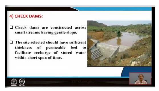
Now fourth is the check dams, check dams are also very important structure, these are constructed across the small streams having gentle slope. So, if the stream is having with gentle slope then check dams are the best structure which can be constructed across the stream. So, the site is selected, this would have sufficient thickness of permeable bed to facilitate recharge of stored water within short span of time.
