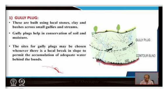
So, the first method through which just the first method which we are generally following for the recharging of the aquifer in rural or in urban areas is the gully plugging. So, this gully plugging, these gully plugs generally are built using the local stones which are available in the village in the urban areas and clay and the bushes across some gullys and streams so small, small gullys and streams remains in the rural areas as well as in urban areas.
