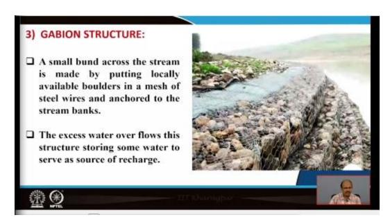
Now next is the gabion structure. So, this is also a very important structure through which the recharge can take place. A small bund but these bunds are made up of available boulders and you can see also some mesh like structure is clear in the figure. This is the mesh of the steel wires which are anchored to the stream banks, so a small bund, it is a small one where across the stream is made by putting local available boulders.
