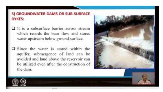
Now next is the groundwater dams or sub-surface dykes. So, dyke is a structure which generally remains embedded in the rocks, so dyke these are the 2 geological terms. It is a sub-surface barrier you can say it is a barrier also, across stream which retards which is control which stops the base flow and stores water upstream below the ground surface. So, we have read about the base flow also when we are discussing about the runoff. So, in this case what is happening?
