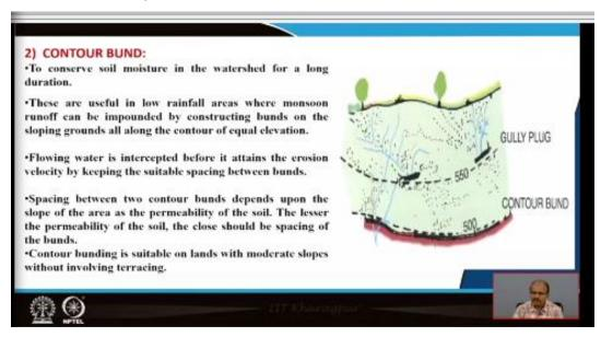
Second is the contour bunding. So, to conserve soil moisture in the watershed for a long duration generally the contour bunding method is being followed. So, this method is following because for the conservation of soil moisture in the watershed for a longer duration. And also these are useful in low rainfall areas where monsoon runoff can be impounded by constructing bunds on the sloping grounds all along the contour of equal elevation.
