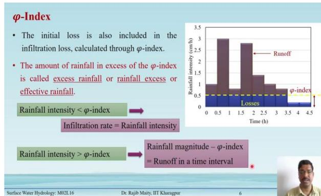
The initial loss is also included in the infiltration loss, calculated through  $\phi$ -index. The amount of rainfall in excess of the  $\phi$ -index is called excess rainfall or rainfall excess of effective rainfall.
