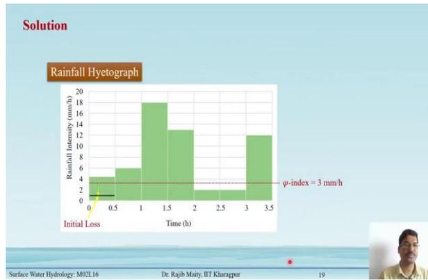
In fig.4 you see that difference in this plot that the initial first part, the initial loss is designated here and this phi index is given as a 3 mm per hour.
