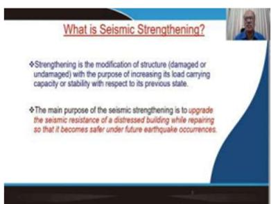
So, basically, what we are trying to answer to that, what is seismic strengthening? When we talk about the term called strengthening, the strengthening is nothing but the modification in the structure that we are trying to address. The structural member could be damaged or undamaged as I said that it could be undamaged but it is deficient in carrying the proper seismic load that is stipulated as of the present criteria or stipulations.
