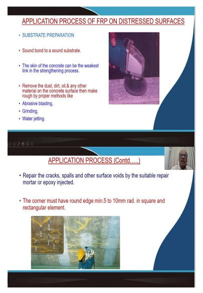
Now, what I am going to discuss with you today here is, how FRP can be applied on the surface or what is the process through which we adopt FRP on the concrete structural element for strengthening the concrete structural member. So, the concrete surface on which we apply FRP we call that a substrate. So, we need to prepare the substrate in an appropriate manner.
