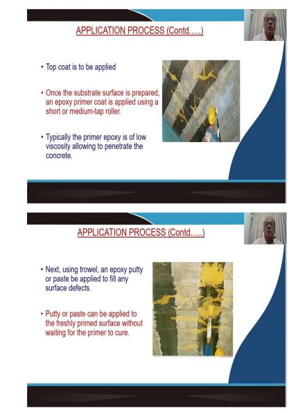
And then subsequently what you need is that onto top of that prepared surface, you will have to apply a coat of epoxy. So, if you have to apply the epoxy primer coat in such a way that if you have finer cracks that epoxy we will penetrate through that and that can be allowed if you use low viscosity epoxy.
