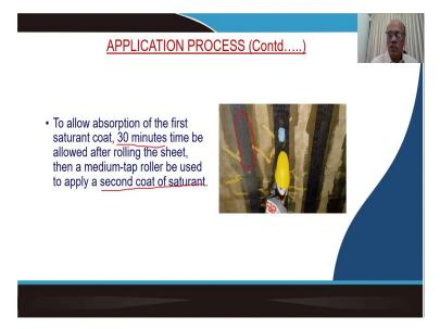
So, first you allow this epoxy to get absorbed and also to penetrate through in the FRP then maybe at around after 30 minutes, what you can do is that you can roll it again and apply a second coat of saturant which is epoxy on this surface. So, you can apply another coat of epoxy and allow these to be cured.
