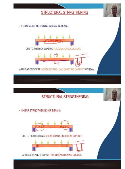
Now, as we were discussing earlier that you get the stresses of different forms in different structural members and we need to strengthen them in an appropriate manner. So, that you get strengthening and here we are using FRP as a material for strengthening. Now, say for example, in a beam.
