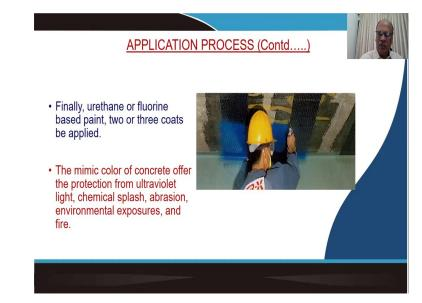
So, after you complete these and after the curing process is completed then you can apply 2 or 3 coats of paints so that the FRP gets protected against ultraviolet rays because in presence of ultraviolet or when it gets exposed to ultraviolet rays, the FRP material normally deteriorates. So, it is better that to prevent these FRPs deteriorations from ultraviolet ray from chemical actions or from environmental actions is better to coat with appropriate paints.
