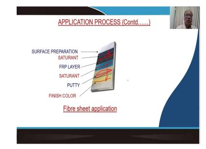
And just to show you different layers that we provide in this FRP system along the thickness you have the substrate you prepare the substrate first to apply the epoxy as a saturant in this then you have the FRP layer then again you provide the saturant that so, that it penetrates through the FRP and then creates a bond between the substrate and the FRP.
