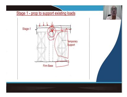
Second thing is that after you place the temporary supports in position, then we try to pay our attention to the column member which is in distress. Now, here as you can see that in the previous case here, you see only this part of the reinforcement was exposed, the concrete got spalled up from there, but in this case.
