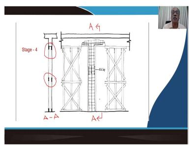
Where, we try to provide some kind of a supporting staging on either side of the column member. So, now, you see this, the side shuttering has been provided, but still you can see the reinforcements from the face. Now, the front reinforcement also I mean front part of the column also has to be provided with a shuttering and this is the side view if I take a section here you will get a view like this.
