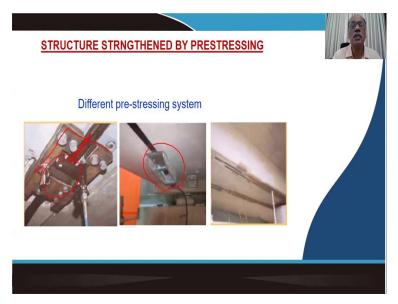
But the different kinds of anchors that are available and that can be put in place are like this as you can see over here it is a kind of a plate which is fixed on the surface of the beam and here you have an arrangement through which the anchor plates or the anchor cables can be taken in and the tensile pull can be applied on to these members.
