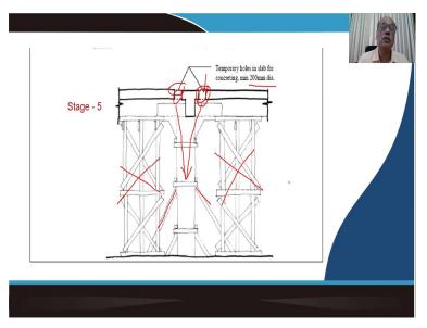
So, in the next stage what we do is that here we provide the shuttering material to the column and to the beam. But once you provide the shuttering naturally all four sides gets covered these are the clamping material that has been provided also in some kind of a temporary support has been given, so that the column member does not get moved or displaced.
