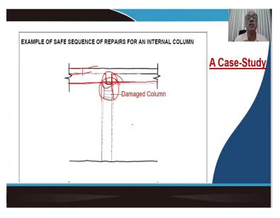
Now, let me talk about a case study, where a beam column junction can be repaired, you see this is a system where this is basically a slab as you can see and this is the bottom part of the slab. So, this is the thickness of the slab and the slab has a beam, this is a beam which is running in the longitudinal direction is a perpendicular to the screen.
