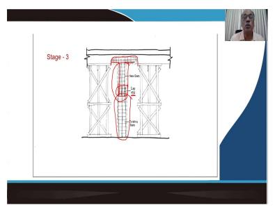
And in the third stage you can see this that you have the existing reinforcement which are there in the column and then we bring in newer reinforcements in this and give a lap of the new reinforcements and the old reinforcements this is the lap zone that has been shown and in comparison, we normally required 40 times the diameter of the bars.
