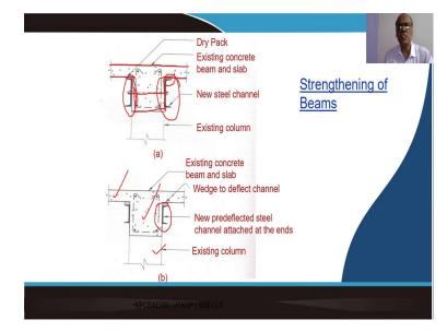
Well, while we talk about the strengthening of beams the reinforced concrete beams obviously, we are talking over here, in this particular case, as you can see here, this is the existing beam, it is a kind of a T-beam, let say it is a part of the slab and this is the beam member again, this is the slab. So, this existing slab beam system is strengthened by using steel channel members on either side as you can see here.
