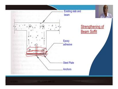
There is another scheme which is adopted over here, as you can see that the bottom fiber the tension zone has been further strengthened by adding a plate at the bottom of the socket of the beam and to have a continuity of this plate, this plate has to be held in position and to hold the plate in position two side plates have been provided, one on this side, on this side and these side plates are getting connected with the bolts.
