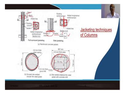
Now, I have spoken about the jacketing of column members earlier in my previous lecture, where I had shown that the concrete members, concrete columns of square or rectangular shapes if they are in distress, how they can be jacketed using either concrete as material or steel as material. And those we have looked into.
