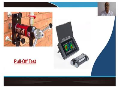
There is another kind of a test which you call as a pull-off test, which gives you the strength of the surface. In this instrument you try to apply a force and try to pull off, and then what is the force that is needed to pull it off, and then you can find out the stress and the corresponding strength of the material or the concrete that you are investigating.
