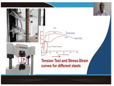
And so is for the reinforcing steel, you cut a sample of the reinforcing steel which from the existing structure, and that bar is hold under the clip with the gauge length, and then if you put in the tensile specimen, you pull this bar to find out that what are the stresses getting generated. I mean, how much extension is happening under the load, or thereby stress versus strain, you can plot it.
