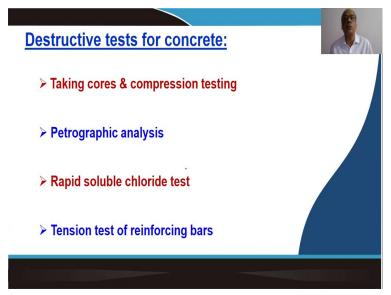
So these are different kinds of tests that you can adopt while going for the nondestructive test. Similarly, there are sets of destructive tests which can be adopted for concrete structural system. And one of the very important destructive test is that we try to extract some core sample from the existing structural elements, and then those cores are tested in a compression testing machine to understand what is the strength of the concrete.
