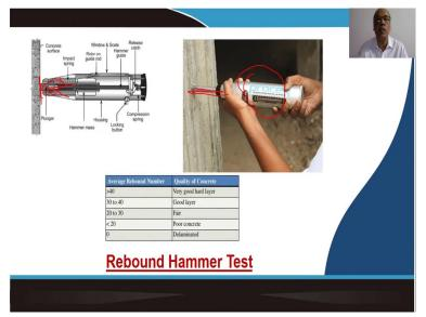
Rebound hammer test is a kind of a test where you can find out the surfacial hardness of the structural system. This is basically, you have a piston or a plunger which moves inside the cylindrical specimen, and is spring loaded. So, this plunger, when it is touched on the surface, and if you try to push and give some energy, impart on the structural system, the structural system rebounds on that impact that you create, and from which you can find out that how hard the surface is.
