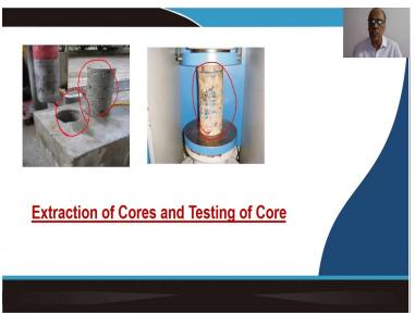
So, here, you can see that this shows how from the structural elements the cores can be extended. There are core cutter of different sizes, of different diameters, and depending on the depth of the concrete element, you get cores. And then this cores are tested under compression testing machine to understand that what is the strength of the concrete.
