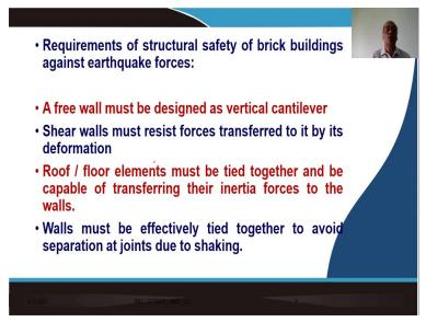
So, if you look into from the safety aspects of the masonry building against earthquake forces, what you should definitely have is that the walls that we get, four walls that you have in the building, these walls are designed when you try to achieve the thickness, when you try to find out the stresses, consider that as a vertical cantilever disregarding the supports that you have. That is of course on the conservative side, that you will be designing the wall as a vertical cantilever.
