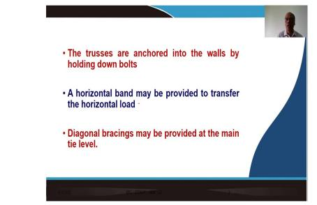
So, what is being said is that the trusses are anchored into the walls by holding down bolts which I have just explained. So, if you want to make a structure resistant against the seismic effect, then, and if you have a masonry system where you have the masonry walls and the roofing is provided with the different kinds of material like GI seatings or other things, then what you need to do is that you need to provide appropriate trusses.
