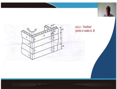
So, you can make use of that kind of a detailing, or sometimes we can go for a detailing of this kind. As I said that corner element could be, may be made out of concrete with some kind of a toothing, and these toothing can be connected with the masonry system, and thereby your corner becomes effective, and thereby the cracks will not be generated.
