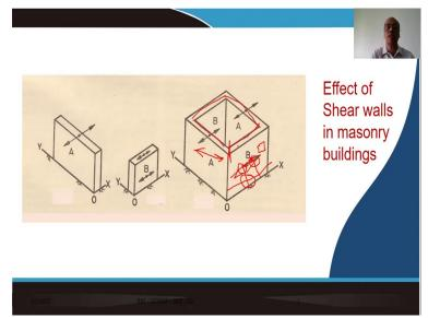
Well, as we have discussing about the masonry structures, we, let us talk about the systems that we see normally in masonry structural systems. Now, here is typically as you can see this is a kind of a box section that we have, and these are the walls. This is one wall, this is a perpendicular wall to this, this is another wall and this is another wall.
