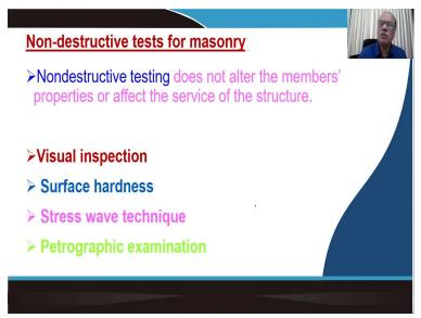
So, we have talked about this. Just to remind you once again that we have spoken about different kinds of tests both in terms of non-destructive as well as the destructive test. Non-destructive test for masonry, normally for any structure for that matter that we do not intervene in the structural system in that sense, we do not disturb the structural system and it does not alter the member properties as such.
