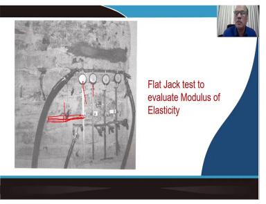
So, having done this test, also as I said that we can find out the modulus of elasticity by applying a particular test which we call as a flat jack test. Now, flat jack test, flat jack is a small instrument which we make use of it. Now, supposing, I cut a slit in a masonry wall, supposing you have a masonry wall and along this you will cut across a slit or you open over an opening.
