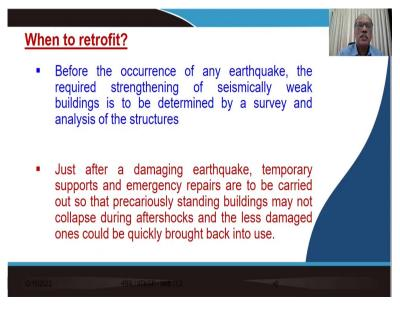
So, the question that counts that when to adopt the retrofit measures and what to retrofit? And as I told you earlier also, that when earthquake happens in an area, because it is you cannot predict beforehand and as a result of all neither you get warning for such earthquakes. Now, when earthquake happens, the structures do undergo damages if they are not designed properly to resist the earthquake of that kind of a magnitude.
