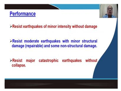
So, what do we expect normally as a performance when we do carry out the seismic design, whether it is a new building, which are designed for the seismic effect, or the building, existing buildings, which are retrofitted or the damaged buildings which are retrofitted? We normally try to adopt these retrofitting measures, the seismic retrofitting measure and there we try to achieve certain performance of those buildings.
