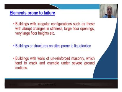
So, just to give you an idea that what kinds of buildings which are seismically weak or where there is a possibility that those structures might undergo damage when they are subjected to earthquake forces. Now, it has been observed from the experience of the past earthquake that buildings with irregular configurations, such as where there is a change, now, the building structure is going with the larger size and then there is a sudden change in the stiffness.
