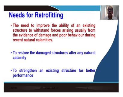
Thereby, the question that come that, what are the needs for the retrofitting or where we tried to adopt it to fitting in the system? The need to improve the ability of an existing structure to withstand forces arising usually from the evidence of damage. As I said that, if you find some amount of distress, damage in the system, you try to repair that damage in a manner where the structure becomes fit to carry the load.
