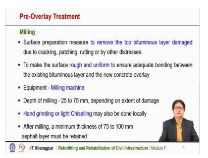
Milling is the surface preparation measure to remove the top bituminous layer damaged due to cracking, patching, rutting or by other type of distress. So, the first step of pre-overlay treatment is to make the surface ready for the paving. So, that can be done by milling. So, by milling, we can remove the top distressed portion of the bituminous surfacing, which are damaged due to cracking, patching or rutting or there may be some other type of distress.
