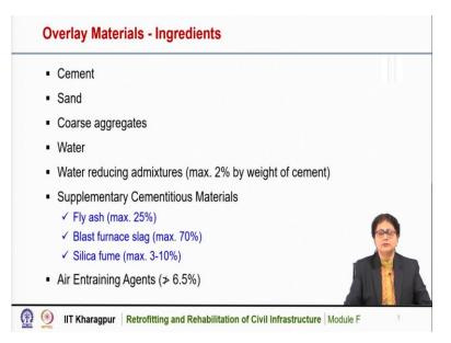
For plain cement concrete or fibre reinforced concrete or high-performance concrete, the ingredients are cement, sand, coarse aggregates, water. So, here also the same ingredients are used. We can also use water-reducing admixtures, maximum 2 percent by weight of cement because we also need to have sufficient workability.
