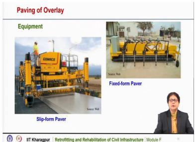
Now we will discuss the paving of the overlay. For paving of concrete overlay, we need to use a paver. Two types of pavers are generally used for the purpose of laying. One is fixed form paper and the other is slip form paver. This is a typical picture of fixed form paper and this is a typical picture of slip form paver.
