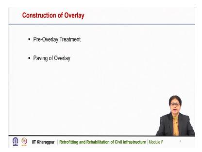
Now for the construction of overlay, there are two broad steps that need to be followed. One is pre-overlay treatment and the other is the paving of the overlay. So, for this type of construction it is important to have a proper pre-overlay treatment. And then we can carry out the paving of the overlay
