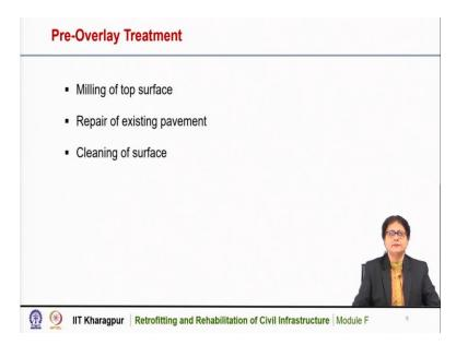
For pre-overlay treatment, there are several steps. One is milling of the top surface, then repairing of the existing pavement and then the cleaning of the surface. So, these are the three steps for pre-overlay treatment or surface preparation.
