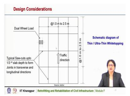
This is a schematic diagram of thin or ultra-thin white topping; here the panel sizes are much less as compared to conventional concrete pavement. In case of conventional concrete pavement, the standard panel size in India is 3.5 meter  $\times$  4.5 meter. Whereas, for whitetopping or thin or ultra thin whitetopping, it is much less maybe 1 meter  $\times$  1 meter or maximum 2.5 meter and to be square or rectangular panels.
