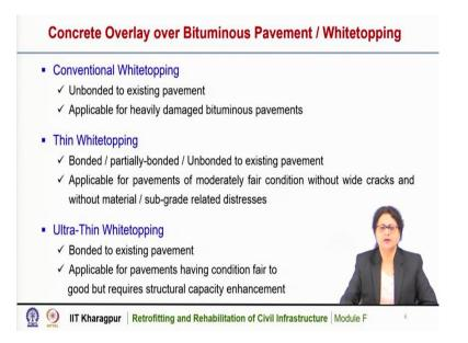
So, we will discuss the concrete overlay over bituminous pavement or whitetopping and as we have just mentioned that it is of 3- types conventional white topping, thin whitetopping and ultra thin whitetopping depending on the bonding condition and their applicability and thickness. So, in case of conventional whitetopping just a recapitulation.
