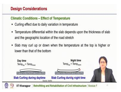
Now, we will discuss the climatic conditions; particularly the effect of temperature, the temperature effect is also significant in case of concrete overlay, there may be curling effect due to daily variation of temperature, temperature differential is there within the slab due to the daily variation of temperature in day time or night time and that depends upon the thickness of the slab and also on the geographical location of the road stretch.
