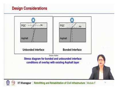
This is the stress diagram for Bonded and Unbonded Interface conditions of overlay with existing asphalt layer. So, here in this case, it is the Unbonded Interface. So, this is the existing asphalt or bituminous layer and this is the concrete overlay. Now, if there is no bonding, then the existing bituminous layer does not contribute anything to the load carrying capacity to the overlay.
