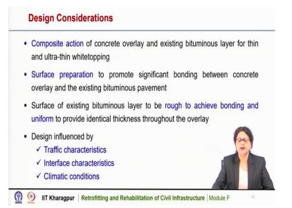
Now for the design consideration the concrete overlay and the existing bituminous layer for thin and ultra-thin white topping, a composite action is taking place. So, the concrete overlay and the bituminous layer behave such that there is a composite action and for this it is important to have a proper surface preparation.
