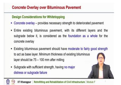
Now, we will discuss the design considerations for whitetopping. Concrete overly provides the necessary strength to the deteriorated pavement. Entire existing bituminous pavement with its different layers and the sub-grade below it is considered as the foundation as a whole for the concrete overlay.
