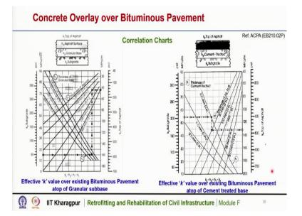
These are the Correlation Charts that has been developed by an (ACPR) American Concrete Pavement Association. This chart gives the effective k value over existing bituminous pavement on top of granular sub base. So, if the existing pavement is shown here, it is schematically shown. So, this is the existing asphalt layer and this is the granular base which is the sub base for this pavement and this is the sub-grade.
