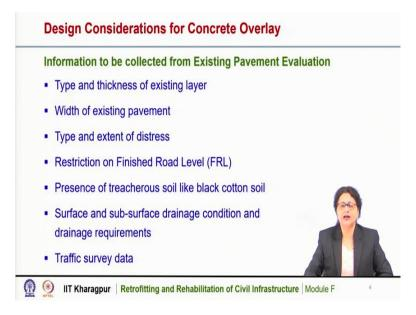
While designing a concrete overlay it is important to carry out pavement evaluation. Pavement evaluation is an important component for any maintenance and rehabilitation work of infrastructure. For pavement therefore, it is also important to carry out a systematic evaluation of the existing pavement and from the evaluation of pavement we can get several informations which are useful for the design of concrete overlay.
