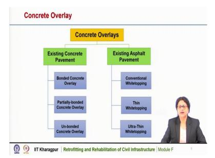
We have discussed in the previous lecture that there may be different types of concrete overlay. For existing concrete pavement, we may have Bonded Concrete Overlay, Unbonded concrete overlay or Partially Concrete Overlay. And in case of asphalt or bituminous pavement, we may have conventional overlay or conventional white topping.
