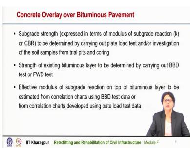
The subgrade strength, which is generally expressed in terms of modulus of subgrade reaction, or CBR to be determined by carrying out plate load test or investigation of the soil samples from trial pits and coring, the strength of the existing bituminous layers to be determined by carrying out Benkelman beam deflection test or falling weight deflectometer test.
