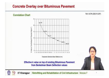
This is a correlation chart developed using Benkelman beam deflection data. So, this is the effective k value that has been plotted in the y-axis and the Benkelman beam deflection data is plotted in the x-axis. So, this gives the correlation between the BBD deflection values and the effective k value on top of existing bituminous pavement.
