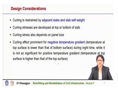
Now, due to variation of temperature, there may be curling effect, but this curling is restrained by the adjacent slabs and the self weight of the slab. So, because of this restraint, there is curling stresses that are developed at the top or bottom of the slab. The curling is restrained by the adjacent slabs as well as by the self weight of the slab.
