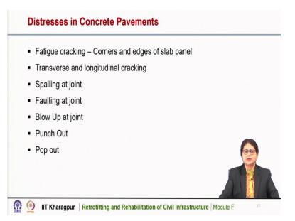
Now, we will discuss the distresses in concrete pavement. Concrete pavement also may have different types of distresses due to loading or environmental effects. The type of distress are fatigue cracking and these cracking's may occur at corners or edges of the slab panels. They may be transverse and longitudinal cracking as well. Joints are the location of distresses sometimes in concrete pavement.
