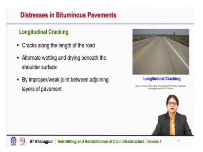
Cracking may be there in bituminous pavement. The cracking may be longitudinal or transverse, this is a typical picture of longitudinal cracking, the cracks are along the length of the road.
