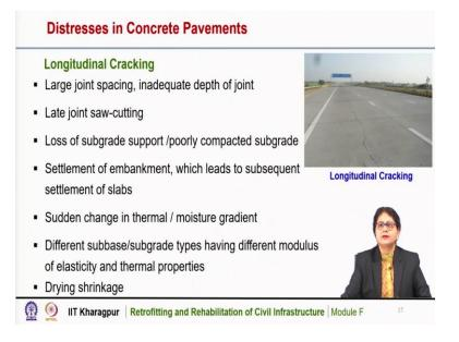
Longitudinal cracking may be also there in case of concrete pavement. This type of cracking may be due to large joint spacing, inadequate depth of joint etc. Generally for concrete pavement, the joints should be placed or saw-cut at regular interval but sometimes if the panel size is quite large, then cracks may appear in between.
