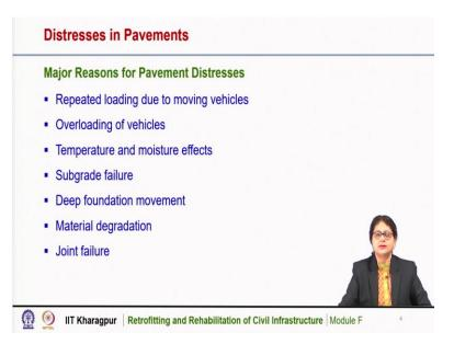
Pavement is a structure that is supported on foundation. The foundation is composed of different layers of base, sub-base and compacted subgrade. And the main load coming on the pavement is the moving vehicular load. Like all other structures, pavement may also get
