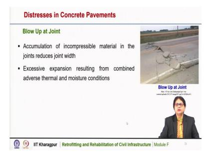
Blow up type of distress is another type of joint related distress in concrete pavement. Here also if the joint is not having adequate width, then due to expansion of the pavement with seasonal increase in temperature, that may cause a collision of the two adjacent panels. So, that results into this type of blow-up type of distress of the pavement.
