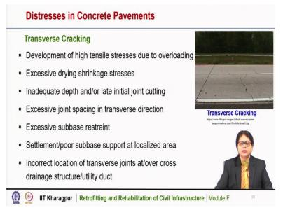
Transverse cracks may also appear in concrete pavement. This is a typical picture of transverse cracking into concrete pavement and these cracks are due to load associated. So, when there are high tensile stresses developed on the pavement due to excessive loading or overloading that may cause cracks on the pavement and it may propagate. So, this type of transverse cracking may appear on the pavement.
