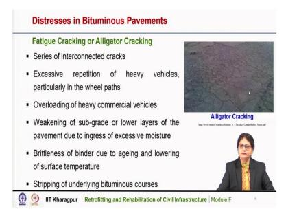
Fatigue cracking or sometimes called alligator cracking is due to the formation of interconnected cracks on the surface of the pavement. So, here is a typical picture of fatigue cracking or alligator cracking, we can see that there are a number of cracks are there and that causes deterioration of the pavement.
