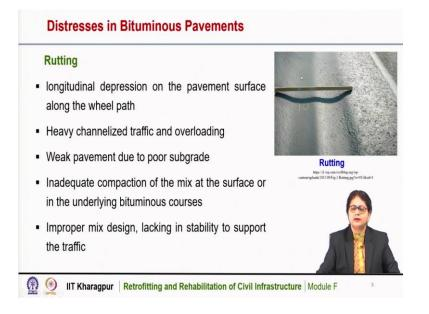
Rutting is also another major distress in case of bituminous pavement, this is also called permanent deformation. It is the longitudinal depression on the pavement surface along the wheel path. So, here we can see that this is a typical picture of rutting and this is along the length of the road the vehicle is moving along this path. So, these are typical wheel paths.
