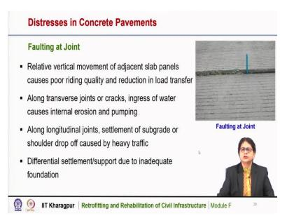
Faulting of joint is also another type of distress in concrete pavement that hampers the functionality of the pavement that means the riding quality is reduced significantly due to faulting of joints. It is the relative vertical movement of the adjacent slab panels that causes poor riding quality and reduction in load transfer.
