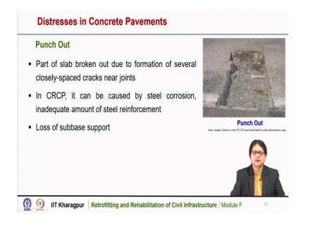
Punch out is another type of distress in concrete pavement and particularly it is seen when the pavement is reinforced. Here this type of distress is found when there are a number of cracks appear on the pavement and in between several cracks, the portion of the slab is broken out and that is shown here if there are a number of cracks on the pavement, that may cause the loss of material within that region.
