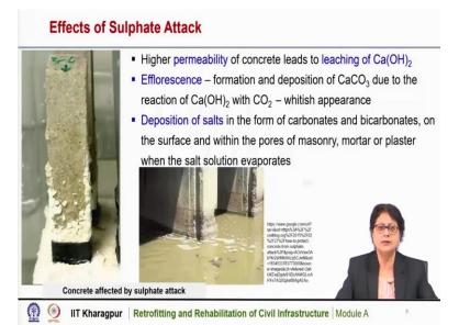
Effect of permeability is also significant in sulphate attack. Higher the permeability of concrete leads to leaching of calcium hydroxide. Calcium hydroxide is the product of hydration and which is present in concrete. And because of the sulphate attack, there may be leaching of calcium hydroxide that leads to formation and deposition of calcium carbonate due to the reaction of calcium hydroxide with carbon dioxide, this is called efflorescence.
