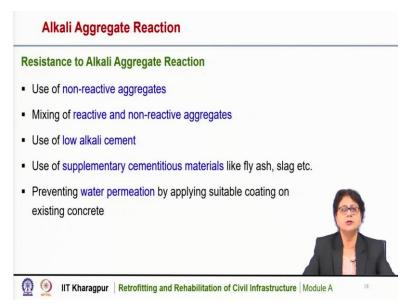
The alkali-aggregate reaction can be resisted with the use of non-reactive aggregates. If in some cases it is unavoidable to use non-reactive aggregates then a mixing of reactive and non-reactive aggregates may reduce the alkali-aggregate reaction in concrete. Use of low alkali cement is also beneficial because the alkali content if it is low, then the reaction also will be less, so the distress also will be less.
