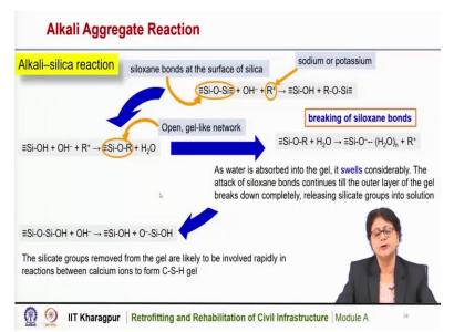
Now, we will discuss the alkali-silica reaction, alkali silicate reaction, and alkali carbonate reaction. In alkali-silica reaction, it is the siloxane bonds at the surface of the silica which is present in aggregate and that is reacting with the alkalis present in the cement paste. So, this is the sodium or potassium denoted by R and this siloxane bond is reacting with the hydroxide ions and alkalis present in the mix to form this Si-OH, this is actually in these reactions.
