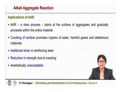
Implications of alkali-aggregate reaction – Alkali aggregate reaction is a slow process, it starts at the surface of the aggregates and gradually proceeds within the entire material. Due to the alkali-aggregate reaction, the cracking of the surface occurs, which promotes further increase of water, harmful gases, and deleterious material and that accelerates further damage. Because of this cracking, the entire surface gets affected and a map cracking type of appearance is formed.
