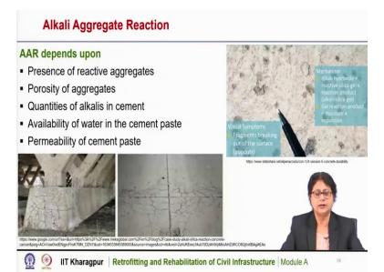
AAR depends on several factors, one, of course, is the presence of the reactive aggregates. Reactive aggregate is the main factor that is responsible for alkali-aggregate reaction. Porosity of aggregate is also another factor that may affect this type of distress, the quantities of alkalis is present in cement because the reactive aggregates react with the alkalis present.
