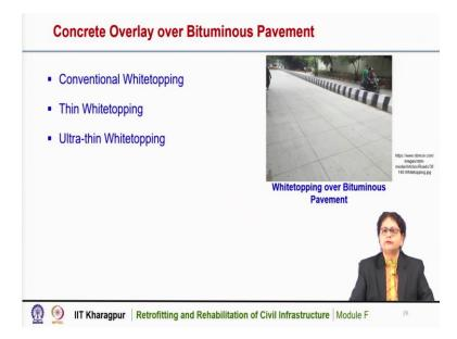
Now, we will discuss the concrete overlay over bituminous pavement. As we have mentioned earlier, there are three types of concrete overlay over bituminous pavement one is conventional white topping, thin white topping and the other is ultra-thin white topping. This is a typical picture of white topping over bituminous pavement.
