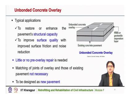
Typical applications for unbonded concrete overlay are to restore or enhance the pavement structural capacity and to improve the surface quality with improved surface friction and noise reduction. So, to improve the strength or structural capacity of the existing member, we can use an unbonded concrete overlay and since it is unbounded, so there is no requirement for pre-overlay repair of the existing pavement.
