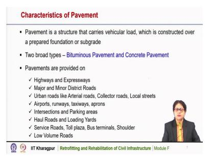
Concrete overlay is applied on pavement. So, here we will discuss very briefly the two broad types of pavement, pavement is a structure that carries the vehicular load which is constructed over a prepared foundation or subgrade. It is not the footpath. So, it is the structural component which carries the moving vehicular load.
