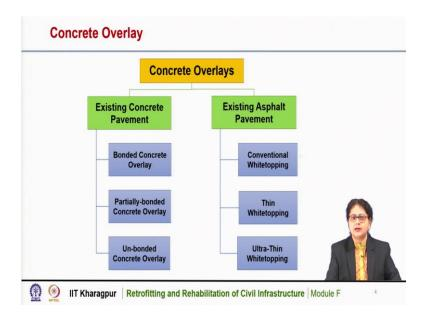
Concrete overlays can be applied for both concrete pavement and asphalt or bituminous pavement, depending on the bonding condition the overlays can be of different types. In case of concrete pavement, the concrete overlay can be of three types, bonded concrete overlay, partially bonded concrete overlay and unbonded concrete overlay.
