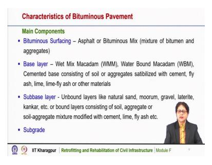
Now, we will discuss very briefly the characteristics of bituminous pavement. The main components are bituminous surfacing, base layer, subbase layer and subgrade. So, the bituminous surfacing is the top layer, it is the asphalt or bituminous mix. The surface layer is composed of bituminous mix, it is a mixture of bitumen and aggregates.
