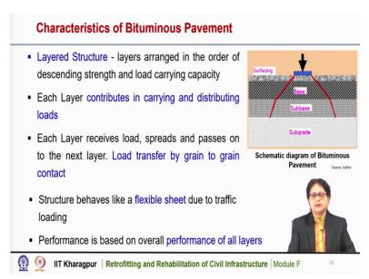
So, the characteristics of bituminous pavement is that it is a layered structure, layers are arranged in the order of descending strength and load carrying capacity. So, the top layer has the maximum strength and as we go down the strength reduces. So, the layers are arranged in the order of descending strength and load carrying capacity.
