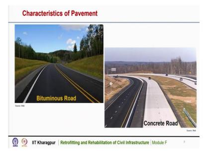
So, these are the two broad types of pavement. One is bituminous pavement or sometimes called blacktop pavement, we can see here that this is a typical bituminous road. The main ingredient is the bitumen which is hydrocarbon and the colour is black. So, the colour of the pavement is also black and this is a picture of concrete road.
