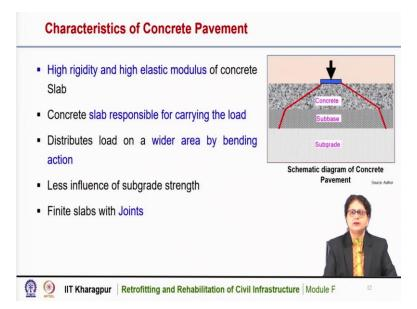
The characteristics of concrete pavement are somewhat different as compared to bituminous pavement. In case of concrete pavement, it is the concrete slab that is responsible for carrying vehicular load. So, the concrete slab is the main component in case of concrete pavement and the load is taken by the concrete slab itself.
