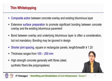
In case of thin white topping, there is a composite action between the concrete overlay and the existing bituminous layer. For thin white topping, it requires extensive surface preparation to promote significant bonding between the concrete overlay and existing bituminous pavement. The bond between overlay and the underlying bituminous layer is often a consideration but not mandatory.
