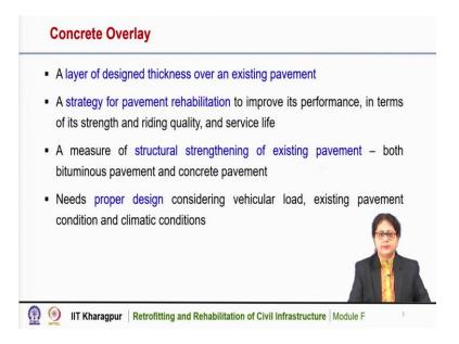
Concrete overlay is a layer of design thickness over an existing pavement. It is a strategy for pavement rehabilitation to improve its performance and service life. The performance is in terms of its structural capacity and also the functional capacity, that is the riding quality and safety. So, it is a strategy for pavement rehabilitation, so that its structural capacity is enhanced as well as its functional capacity is improved.
