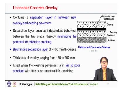
In case of unbonded concrete overlay, it contains a separation layer in between the new overlay and the existing pavement. So, a separation layer is to be provided and that creates the unbonded condition between the new overlay and the existing pavement. This separation layer ensures independent behaviour between the two slabs, thereby minimising the potential for reflection cracking.
