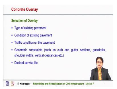
Now, we will discuss that how we can select an overlay. What are the parameters that govern the selection of overlay? It depends significantly on what type of the existing pavement is, whether it is a bituminous pavement or it is a concrete pavement, these are the two broad classifications of pavement there could be different other types and depending on where the pavement is situated, that also governs the type of overlays selection.
