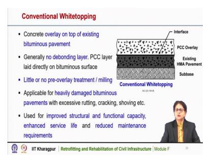
Now, we will discuss this in detail. Conventional white topping is the concrete overlay on top of existing bituminous pavement. It is generally having no debonding layer, the PCC layer is laid directly on the bituminous surface, little or no pre-overlay treatment is required or we can do a milling of the existing surface. It is applicable for heavily damaged bituminous pavement with excessive rutting, cracking, shoving etc.
