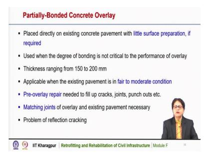
In case of partially bonded concrete overlay, the overlays to be placed on the existing pavement and the existing pavement may require a little surface preparation. It may be placed
