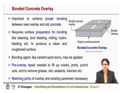
In case of bonded concrete overlay, it is important to achieve proper bonding between the new overlay and the old concrete. And that requires proper surface preparation so that proper
