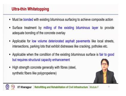
Now, ultra-thin white topping must be bonded with the existing bituminous surfacing to achieve the composite action, in case of conventional white topping bonding is not necessary, in case of thin white topping bonding may be done or we cannot, we may not use bonding, but in case of ultra-thin white topping bonding is a must.
