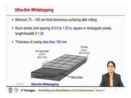
Here also after surface treatment or after milling, the minimum thickness of the bituminous surfacing is 75 to 100 millimetre, we can provide more but minimum this much thickness is required. In case of ultra-thin white topping, we may have even much shorter joint spacing as compared to thin white topping.
