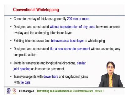
Conventional white topping has thickness generally in the range of 200 millimetre or more because it is designed as a new pavement. It is designed and constructed without consideration of any bond between the concrete overlay and the underlying bituminous layer. The existing bituminous surface behaves as a base layer to the conventional white topping.
