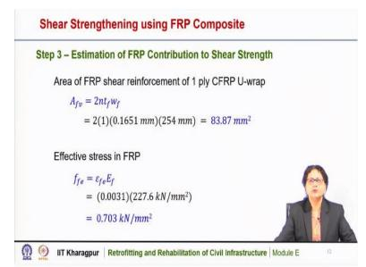
Now, the next step is the estimation of the FRP contribution to shear strength. So, for that we need to find out that what is the area of FRP shear reinforcement for 1 ply of CFRP U-wrapping, so  $A_{fv}$  that is the area of the CFRP is equal to  $2nt_fw_f$  and this also have been discussed in the previous lecture, while discussing the design approach.
