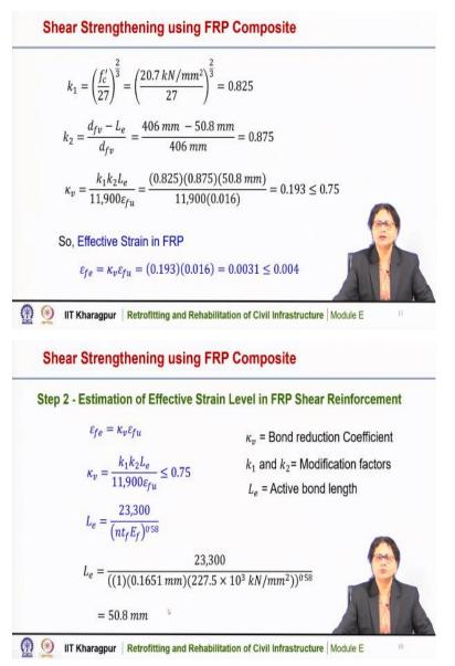
Now, we need to calculate those modification factors this  $k_1$  is just mentioned that it is due to the concrete strength. So, this equation has been developed to determine this modification factors and these equations have been developed based on a number of experiments as we have discussed. So,  $k_1$  is to be found out from this equation and by putting the values of  $f_c$  that is the compressive strength of concrete we can find the value of  $k_1$  as 0.825.
