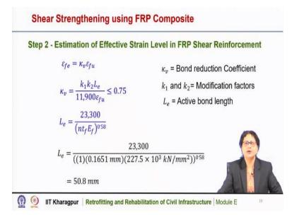
Now, the next step is the estimation of effective strain level in the FRP shear reinforcement and for that we have to use this equation  $\varepsilon_{fe} = \kappa_v \varepsilon_{fu}$ ,  $\varepsilon_{fu}$  is the design strain and that we have just obtained by multiplying the ultimate strain into the environmental reduction factor and  $\kappa_v$  is the bond reduction coefficient.
