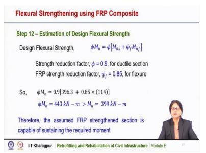
Now, we have to estimate the design flexural strength. So, the design flexural strength is given by this equation and this also was mentioned in the previous lecture. So,  $\phi M_n = \phi M_{ns} + \psi_f M_{nf}$ ,  $\phi$  is the strength reduction factor and for ductile section the value is 0.9 as given in the ACI guideline. And for the FRP we need to use another strength reduction
