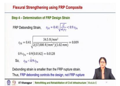
Now, after knowing the strain at the bottom of the concrete at the time of FRP installation we need to determine the FRP designs strain. Now, the FRP design strain we have to calculate first the FRP debonding strain and this debonding strain can be obtained from this equation, we discussed this that there may be different types of failure for an FRP strengthened member, it could be due to concrete crushing or it could be due to rupture of FRP or it could be due to debonding.
