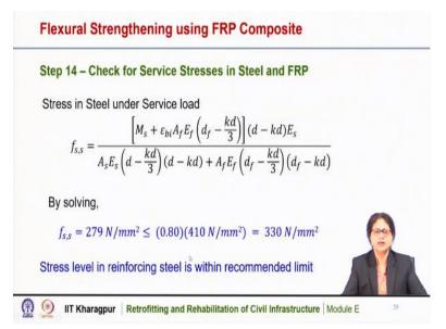
So, we can find out the service stresses in steel and FRP by knowing the value of kd. So, the stress in the steel under the service load condition is given by this equation, this also we have discussed in the previous lecture. So, this is the equation for estimating the stress in steel under the service load condition so that is coming out as 279 by putting the values.
