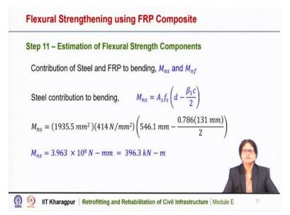
Now, we have to estimate the flexural strength components, the strength will be taken by the steel as well as the FRP. So, the contribution of steel and FRP to bending we have to calculate. So, the contribution of steel is written as  $M_{ns}$  and the contribution of FRP is  $M_{nf}$ .
