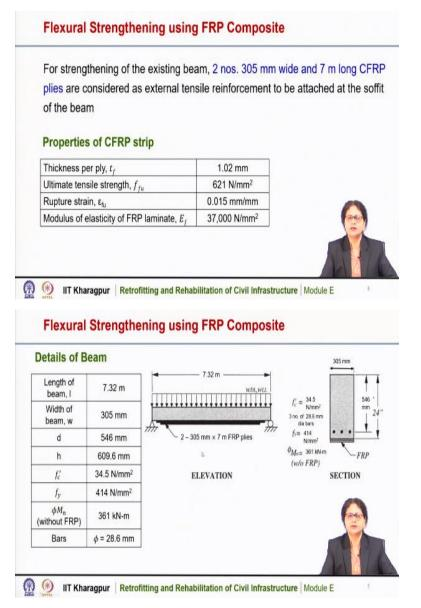
Now, we need to strengthen it with FRP composite for strengthening of the existing beam 2 numbers of 305 millimeter wide and 7-meter long CFRP sheets are considered as external tensile reinforcement and that is to be attached at the soffit of the beam. So, here in this diagram also it is shown that we are considering 2 FRP plies of 7-meter length and they are of full width. So, they are of width 305 millimeter and that needs to be attached at the bottom of the beam for flexural strengthening.
