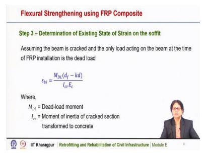
Now, we need to determine the existing state of strain on the soffit of the beam. Assuming the beam is cracked and the only load acting on the beam at the time of FRP installation is the dead load. We have mentioned in the previous lecture that we need to estimate also the epsilon bi, which is the strain of the concrete at the soffit during the time of FRP installation.
