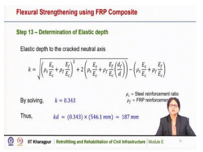
Now, we need to check the serviceability criteria and for that we need to determine the elastic depth. So, elastic depth to the cracked neutral axis has been given by this equation and we have to calculate the depth of neutral axis for the elastic condition and that is kd. Here  $\rho_s$  is the steel reinforcement ratio and  $\rho_f$  is the FRP reinforcement ratio. So, k can be estimated using this relationship, so by solving we get k is equal to 0.343 thus kd is equal to 187 millimeter.
