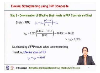
Now, we will determine the effective strain level in the FRP, concrete and steel. So, we have discussed this, the internal stress strain distribution in the beam. So, from that we have discussed that the strain in the FRP can be written as  $\varepsilon_{fe} = \varepsilon_{cu}[(d_f - c)/c] - \varepsilon_{bi}$ .
