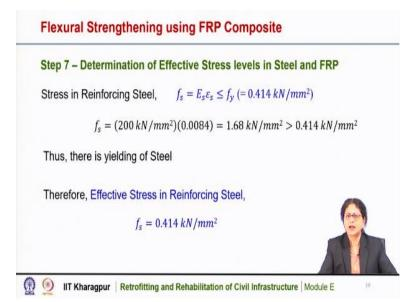
Now, in the next step we will determine the effective stress levels in steel and in FRP. Stress in the reinforcing steel can be written as  $f_s = E_s \varepsilon_s$  that is the elastic modulus of steel into the strain in steel and that should be less than equal to  $f_y$  that is the yield strength of steel.
