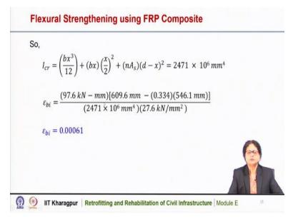
Now, this crack moment of inertia, we can calculate using this relationship and that is coming out as  $2471 \times 10^6$  millimeter<sup>4</sup>. So, we can get I<sub>cr</sub> and from that now we can get the strain in the concrete soffit at the time of FRP installation using this equation  $\varepsilon_{bi}$ . So, knowing the dead load moment and the depth and the kd and the I<sub>cr</sub> also the E<sub>c</sub> we can find out  $\varepsilon_{bi}$ , which is coming out as 0.00061.
