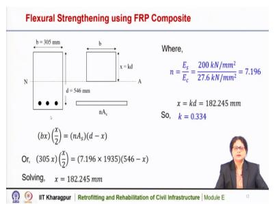
So, considering the cracked section as we can see here this is the beam section and considering the cracked section, we can find out that this is the neutral axis and by considering the moment equilibrium we can write this equation and the modular ratio that is the ratio of the elastic modulus of steel and concrete that is n is calculated here as 7.196.
