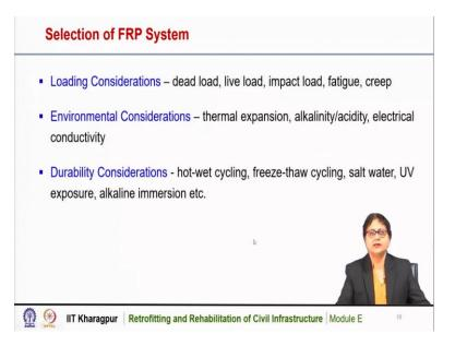
Now, while selecting the FRP system for an existing structure to its strengthening, we have to consider the loading. So, loading consideration should be there. Environmental considerations are also another thing we have to consider. And durability considerations. So, while selecting the FRP system, we have to consider the load coming on the structure, the environmental conditions and the durability conditions or the exposure conditions.
