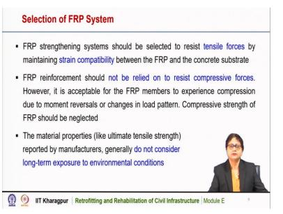
Now, we have to select an FRP system considering the load coming on it. The increase in load is there on the structure, so because of that, it has to carry a higher load and that is why it is to be strengthened. The FRP strengthening system should be selected to resist tensile forces by maintaining strain compatibility between the FRP and the concrete substrate. FRP has excellent tensile strength and tensile modulus therefore, it is used to resist tensile forces only.
