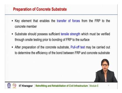
So, for the preparation of concrete substrate, we should follow certain steps. The key element that enables the transfer of force from the FRP to the concrete member. So, the concrete substrate is the key element that enables the transfer of forces from the FRP to the concrete member. So, it is important to prepare the concrete surface properly.
