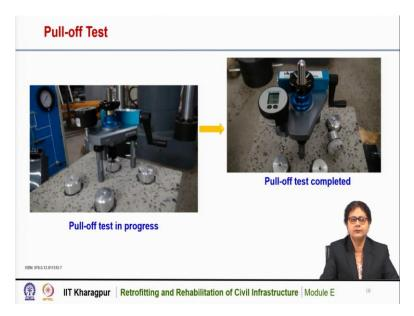
This is the picture of pull out test in progress. We can see that this is the equipment limpet that is used. And these are the aluminum plates which are used for carrying out the test. And
