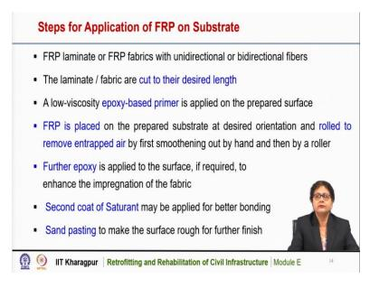
Now, we will discuss the different steps for application of the FRP on the prepared substrate. FRP is available as laminate or fabric with unidirectional fibers or with bi-directional fibers. The laminate or fabric, if it is available, either in rolls or as plates that needs to be cut to their desired length for the application.
