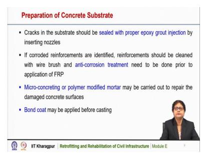
Cracks in the substrate, if they are present that should be sealed with proper epoxy grout injection by inserting nozzles. We have discussed that how the epoxy grouting injection can be done. So, here also before putting the FRP, if the cracks are there, that should be sealed with proper epoxy grouting injection.
