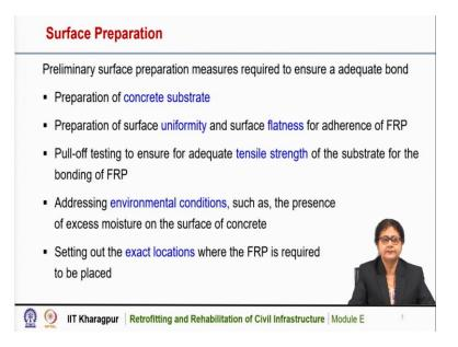
Preliminary surface preparation measures are required to ensure an adequate bond from the FRP to the existing concrete member. So, we need to prepare the surface properly. So, that adequate bond is achieved and the potential of the FRP is achieved. So, the steps are preparation of the concrete substrate. Then preparation of the surface uniformity and surface flatness for adherence of the FRP composite.
