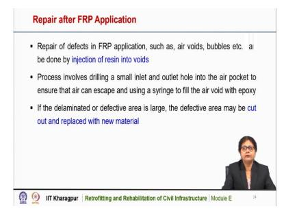
So, if that type of delamination or defect or air void or bubbles are visible on the surface, after installation, then a repair measure is necessary. So, repair of defects in the FRP application can be done by injection of resin into the voids. So, if voids are visible or bubbles, air bubbles are visible then we can use epoxy injection so that the voids are filled up.
