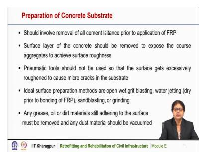
Preparation of concrete substrate should involve removal of all loose materials, cement laitance, etcetera prior to application of the FRP. Surface layer of the concrete should be removed to expose the coarse aggregates to achieve surface roughness. And that gives a better bonding.
