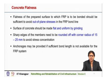
The concrete surface should be flat and that has to be done. Flatness of the prepared surface to which FRP is to be bonded, should be sufficient to avoid out of plane stresses in the FRP bond line. The surface of concrete should be made flat and uniform by grinding. Generally, grinding is used or we can use other methods.
