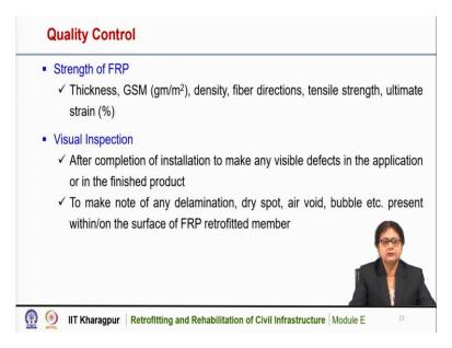
For the FRP, we can carry out several tests to determine the tensile strength, the ultimate strain, the tensile modulus of the FRP, the thickness, the GSM that is gram per meter square of the FRP, the density, the fiber directions generally are given by the manufacturer. However, it is always desirable to test the FRP to determine its tensile strength and modulus values. And also, we can carry out a visual inspection after the installation of FRP.
