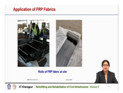
These are the pictures of the application of FRP fabrics on existing concrete members. These are the roles of FRP fabric at site. Here, we can see that these are the carbon fiber reinforced polymer composites. We can see here that they are generally black in color and available in roles. And this is also another picture of the FRP composite. And this picture we have taken from a site where an ROB is being retrofitted with carbon fiber composites. So, these are the roles of FRP fabric at site.
