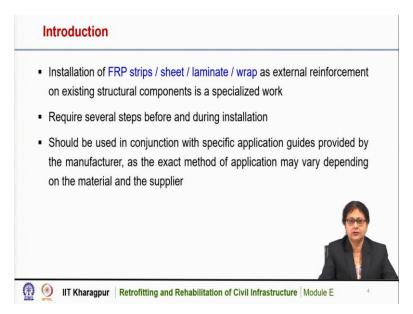
Installation of FRP strips or sheets or laminates or wraps, as external reinforcement on existing structural component is a specialized work. FRPs are generally available as rolls or strips or plates or laminates of different sizes. It may be pultruded or hand layup and those materials are used for the retrofitting purpose of existing structures.
