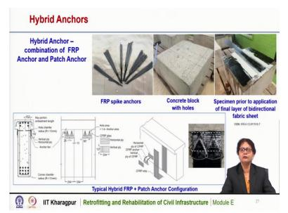
This is a hybrid anchor. And it is actually a combination of FRP anchor and patch anchor. So, here is the FRP anchor with these spikes or fans and dowels. So, this is the FRP anchor and along with this we can use patch anchor. So, this is a concrete block and here first this type of FRP anchor is placed for improving the bond between the FRP laminate and the concrete.
