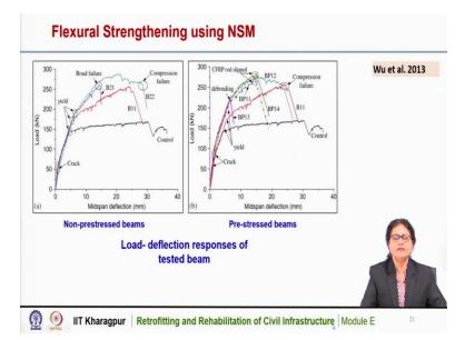
These are the responses of the tested beams; this is for non-prestressed beams and this is for prestressed beams. So, this plot shows that this is the response of the control beam and these are the responses of the non-prestressed beam. So, in all cases, it has been seen that there is a significant improvement of the load carrying capacity of the NSM strengthen beams, we can see here that there is a significant improvement as compared to the control beam.
