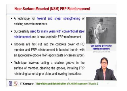
Near surface mounted technique is suitable for improving the flexural and shear strengthening of existing structural members. The technique is successfully used for many years with conventional steel reinforcement, and now, it is used with FRP reinforcement. In this technique, the grooves are cut into the concrete cover of reinforced concrete members. And then, FRP
