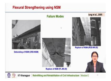
These are the failure modes of the beams that are tested by these experiments by the researcher Jung et al., in 2005. Here it shows that there is debonding of the NSM. This is without Anchorage System. So, here the NSM bars were placed and with increasing load the beam fails due to debonding of the NSM. So, clearly it is shown that there is debonding of the NSM bars. The system with anchorages, the NSM with anchorages here the failure was due to rupture of the NSM.
