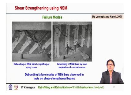
These are some other type of failure modes as observed by other researchers De Lorenzis and Nanni in 2001. Here also we can see those different types of debonding failure occurred in case of NSM retrofitted members. Here we can see that the debonding of the NSM bars by splitting of the epoxy cover. So, these are the NSM bars and the failure is due to splitting of the epoxy cover over these bars.
