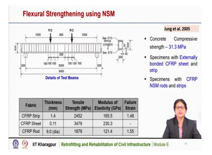
Now, there are different types of investigations on NSM and recently different types of investigations have been done to understand the complex behaviour of the NSM system. So, NSM is an efficient technique for improving the flexural capacity of the members to understand the different parameters on the load displacement responses of the NSM strengthen members, different experiments and analytical works have been done by the researchers.
