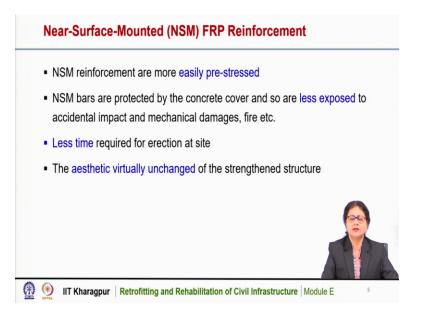
NSM reinforcements are more easily pre-stressed. So, this is also another advantage for NSM, retrofitted members. NSM bars are protected by the concrete cover and so, are less exposed to accidental impact and mechanical damages, fire etcetera. Since they are covered with some amount of epoxy or cement grouting. So, they are not exposed like the strips placed on the existing members.
