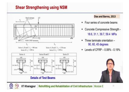
Dias and Barros in 2013 carried out extensive experiments considering different parameters of NSM retrofitted members. Here four series of concrete beams were tested. Series A B C and D and these were T beams, different compressive strength of concrete was used 18.6 to 59.4 MPa and the NSM was also of different types.
