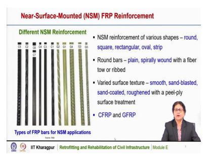
There are different types of NSM reinforcement that are used for this purpose. NSM reinforcement maybe of various shapes, round, square, rectangular oval or strip. So, mostly the round bars are available, but we can also use square bars or rectangular bars, even strips or if FRP plates can be used as NSM reinforcement. Here is the typical picture of the different types of FRP bars for NSM applications.
