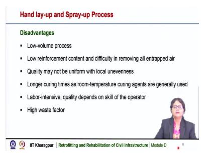
However, there are some limitations; the main disadvantage is that it is a low volume process. If we want to prepare a large number of FRP materials, this hand lay-up or spray-up process is not very suitable, because it is a manual process. So, a lot of time will be required for that. So, this is not very suitable when we require large number of products to be prepared.
