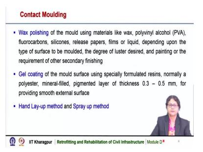
Now, after preparing the mould, the mould need to be wax polished and that can be done like materials, wax or polyvinyl alcohol, fluorocarbon, silicones, etc. And that wax polishing is required to get a uniform finish to the surface. Depending upon the type of surface to be moulded we can select the wax material and also depending on the degree of luster desired and the painting we can use the wax polishing material.
