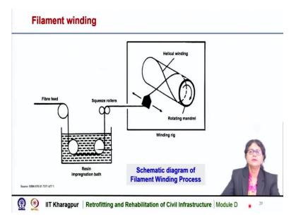
Here is the schematic diagram of filament winding process. This is the fiber to be fed, the fiber is going through this resin impregnation bath. So, it is saturated with resin and then it is squeezed and then it is coming to the winding rig and this is the mandrel. This is the mandrel which is rotating and the fibers are placed onto the mandrel and the winding is helical in nature. And by the rotation of this mandrel, we can have the fibers on it and we can get the product.
