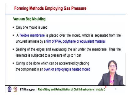
In vacuum bag moulding, only one mould is used. So, unlike the match dye moulding, here only one mould is used. A flexible membrane is placed over the mould, which is separated from the uncured laminate by a film of PVA, polythene or any equivalent material. So, here one mould is used and we are using a flexible membrane placed over the mould.
