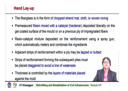
In hand lay-up method, the fiberglass that is used is in the form of chopped strand mat, cloth or woven roving, the resin is used and it has to be pre measured mixed with a catalyst or hardener that is to be deposited on the mould and which is gel coated and wax finished and on a previous ply of impregnated fibers. Initially it has to be on the mould and then some fibers may be there and we can put the resin onto it.
