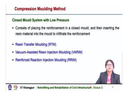
Another method of compression moulding is by using low pressure. So, here it is the closed mould system with low pressure that consists of placing the reinforcement in a closed mould and then inserting the resin material into the mould to infiltrate the reinforcement. So, here we are using a mould and that is a closed chamber. So, that is called closed mould and then the inserting the resin material into the mould to infiltrate the reinforcement that is the fibers.
