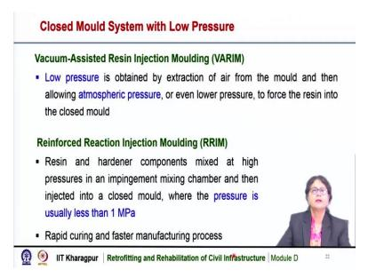
In vacuum assisted resin injection moulding or VARIM that also uses low pressure and this low pressure is obtained by extraction of air from the mould and then allowing the atmospheric pressure or even a lower pressure to force the resin into the closed mould.
