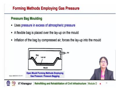
Another one is pressure bag moulding. In this method we are using pressure in excess of atmospheric pressure. Here also a flexible bag is placed over the lay-up on the mould, this is the mould we can see here on the schematic diagram, this is the mould and a flexible bag is placed over the lay-up on the mould. Inflation of the bag is done by compressed air forcing the lay-up into the mould.
