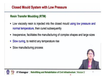
And resin transfer moulding, here we are using low viscosity resin and that resin is injected into the closed mould using low pressure and normal temperature and then it is cured subsequently and slowly. The method is inexpensive, it facilitates the manufacturing of complex shapes and large sizes. The process involves slow curing because it is at the normal temperature and at low pressure.
