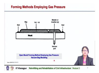
So, here is the schematic diagram of the open mould forming method employing gas pressure that is the vacuum bag moulding. So, here this is the mould, this is the one mould that is used and this is the membrane and the edges are filled, the material is placed here, the edges are filled and the air is evacuated through this vacuum port and with this there is compaction of the material and we can get the FRP product.
