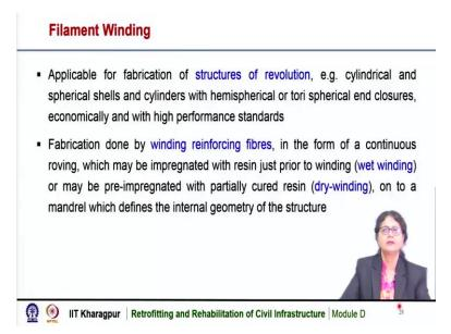
Another technique of FRP manufacturing is filament winding. Filament winding is applicable for the fabrication of structures of revolution like the cylindrical members or spherical members or spherical shell or cylinders with hemispherical, or tori spherical enclosures etc. So, filament winding is a high-performance method and we can get material of FRP with high quality and thus it is economical as well, because we are getting a good quality FRP material from this filament winding method.
