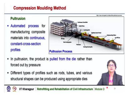
Now, another compression moulding technique is pultrusion. This is an automated process, where the manufacturing composite materials are continuous or constant cross section profiles. So, in case of pultrusion this is much advanced process of manufacturing of the FRP
