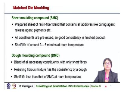
So, the feed material may be sheet moulding compound or Dough moulding compound. In sheet moulding compound, the prepared sheet of resin fiber blend contains all our additives like curing agent, release agent, pigments etc. All the constituents are pre-mixed, so, we can get a good consistency in the finished product and the shelf life is also high in about 3 to 6 months at room temperature.
