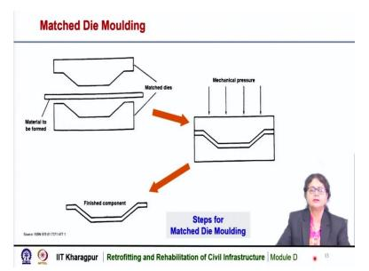
This is the schematic diagram of matched dye moulding process; we can see here. These are the 2 matched dyes. So, this is the mould which is called matched dies and this is the material that is to be formed.
