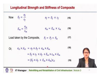
Now, the elastic modulus can be written as stress by strain, so, for the fiber  $E_f = \sigma_f / \varepsilon_f$ . So,  $\sigma_f = E_f \times \varepsilon_f$ , for the matrix  $E_m = \sigma_m / \varepsilon_m$  or  $\sigma_m = E_m \times \varepsilon_m$ .
