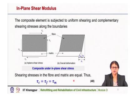
Now we will derive the in-plane shear modulus of the composite. The composite element is subjected to uniform shearing and complementary shearing stresses along the boundaries. So, here this is the composite, similarly, the two phases are shown separately or idealization so this is the fiber part and this is the matrix part, and it is subjected to shear force. You can see here shear stresses are shown.
