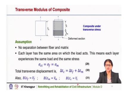
Now, we will determine the transverse modulus of composite. To determine the transverse modulus composite here also we will have some assumptions. The first assumption is that there is no separation between the fiber and the matrix, and the fiber composite is subjected to a transverse loading. As we can see here, this is also an idealized schematic diagram of the composite, the two phases the fiber phase and the matrix phase are denoted here and this composite is under transverse loading.
