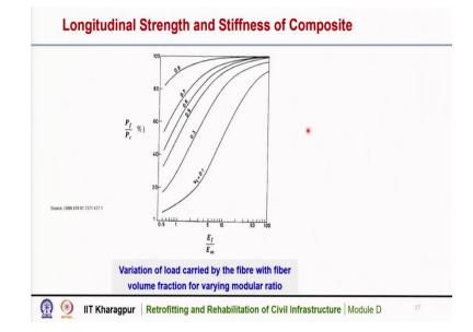
This is a graph that shows the variation of the load carried by the fiber with different fiber volume fraction for wearing modular ratio. So, this graph shows that when the  $E_f / E_m$  is very same, different same 1 to 100 or so, and these are the different fiber volume fraction. So, what is the load shared by the fiber?
