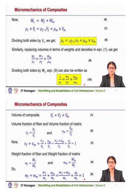
Now, the total weight of the composite is the total weight of the fiber plus the total weight of the matrix. So, we can write the weight in terms of density and volume.
