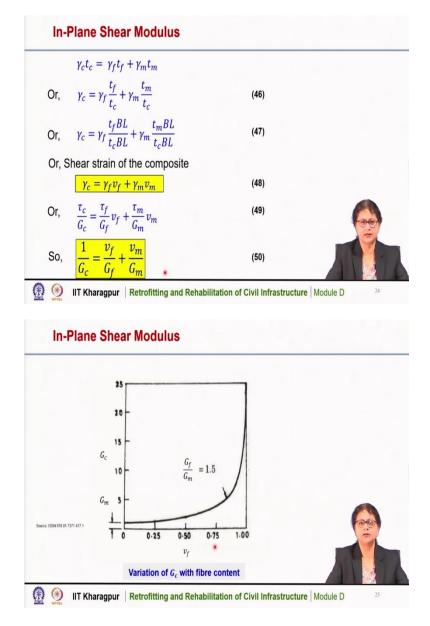
This graph shows the variation of  $G_c$  with fiber content here in the x axis  $V_f$  is plotted and this is the  $G_c$ . Now, with increase in fiber volume fraction the  $G_c$  also increases. So, initially
