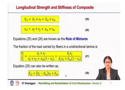
So,  $E_{cl} = E_f \times v_f + E_m \times v_m$ . This equation can also be written as  $\sigma_{cl} = (\sigma_f \times A_f / A_{cl} + \sigma_m \times A_m / A_{cl}) = (\sigma_f \times v_f + \sigma_m \times v_m)$ .
