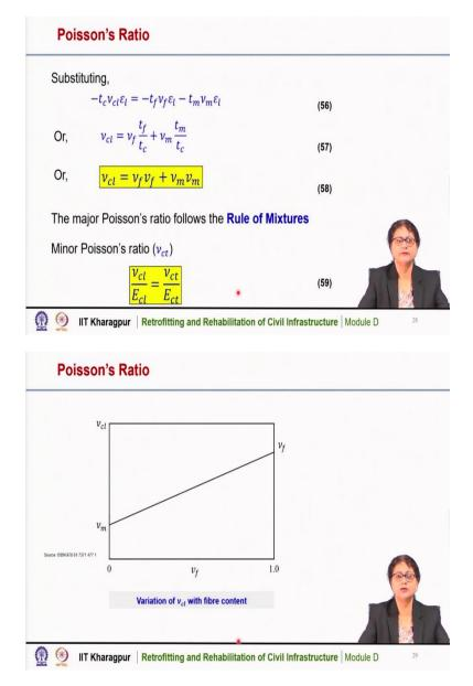
This is the variation of the Poisson's Ratio the major Poisson's Ratio of the composite with fiber content. Here this is the fiber content is plotted in this axis and this is the Poisson's
