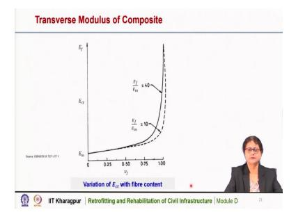
This graph shows the variation of the elastic modulus of the composite in the transvers direction with fiber content. The fiber content are plotted in the x axis and this is the  $E_{ct}$  for different  $E_f / E_m$  values, so we can see here that at lower values of the volume fraction of fiber, there is not significant increase in the transverse modulus of the composite.
