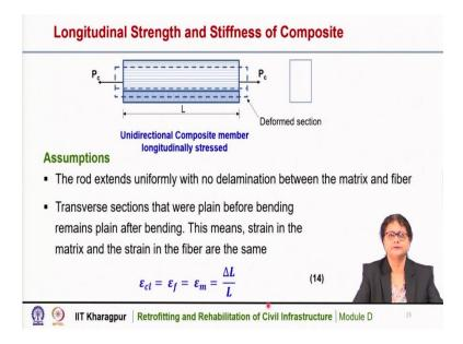
Now, we will discuss how to determine the elastic modulus of the composite along the direction of the fiber. So, it is the longitudinal strength and stiffness of the composite, and it is along the direction of the fiber. So, here is an idealized schematic diagram. This is a unidirectional composite member. We can see here the two phases are shown differently. This is the fiber phase and this is the matrix phase.
