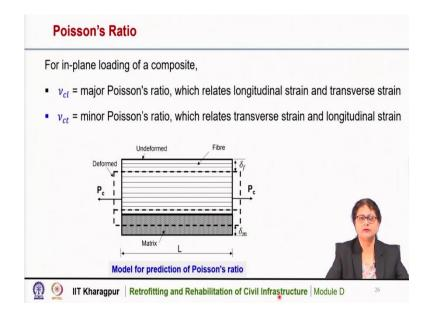
Now, we will discuss the Poisson's Ratio of the composite. For in-plane loading of a composite we have two Poisson's ratio for the composite. One, is the major Poisson's ratio which is denoted as  $v_{cl}$ , which relates the longest eternal strain and the transverse strain. The other one is the minor Poisson's Ratio, which is denoted as  $v_{ct}$ , which relates the transverse strain and the longitudinal strain.
