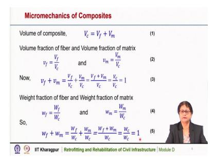
Now, the volume of composite that is  $V_c = V_f + V_m$  that is the volume of fiber plus the volume of matrix. And we have assumed that there is no void, so the volume of composite is the summation of the volume of fiber and the volume of matrix. Now, the volume fraction of fiber and the volume fraction of matrix is written as this. Small  $v_f$  is the volume of fiber by the volume of the composite.
