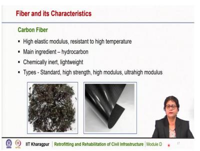
Carbon fiber is also very popular for its wide application; the main ingredient for carbon fiber is hydrocarbon. It has high elastic modulus and it is resistant to high temperature that
