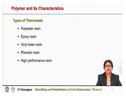
There are different types of thermosets, polyester resin, epoxy resin, vinyl ester resin, phenolic resin and high-performance resin.
