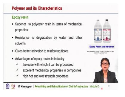
Epoxy resin is another type of polymer which is superior to polyester resin in terms of mechanical properties. It is resistant to degradation by water and other solvents. And it gives better adhesion to reinforcing fibers. The advantages of epoxy resin in industry are the ease with which it can be processed. It has excellent mechanical properties in composite and it is of high hot and wet strength properties.
