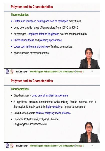
Thermoplastic are materials which softens and liquefies on heating and can be reshaped many times. So, we can heat a thermoplastic and then we can again use it by reshaping it. It is used over a wide range of temperature from 100 degrees centigrade to 300 degrees centigrade. Thermoplastic have several advantages like improved fracture toughness over the thermosetting plastics and it is chemically inert and also has pleasing appearance.
