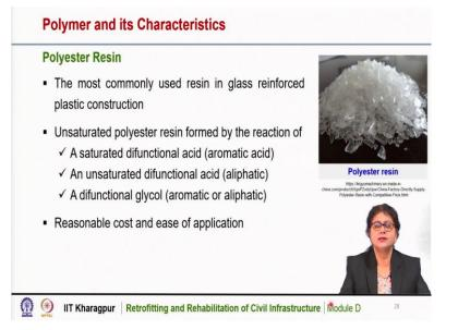
Polyester resin is the most commonly used resin in glass reinforced plastic construction. The unsaturated polyester resin is formed by the reaction of three different types of materials, one is saturated difunctional acid, which is an aromatic acid, another is unsaturated difunctional acid, which may be aliphatic acid.
