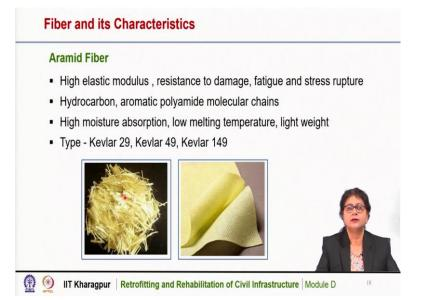
Aramid fiber is also used, the main ingredient for aramid fiber is hydrocarbon and it is the aromatic polyamide molecular chains. So, it consists of hydrocarbon which is aromatic polyamide molecular chains. Aramid fibers also have high elastic modulus and it is resistance to damage fatigue and stress rupture. It is of high moisture absorption value and low melting temperature and it is also lightweight.
