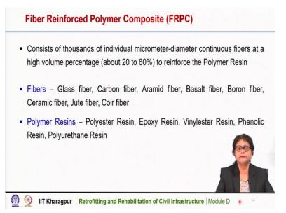
Now we will tell you that, what is a fiber reinforced polymer composite or FRPC. Fiber reinforced polymer composite consists of thousands of individual micrometer-diameter
