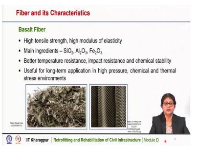
Basalt fiber is also used recently and it also has high tensile strength and high modulus of elasticity. In recent years in retrofitting work also, basalt fiber has started its application, the main ingredient of basalt fiber is the silica, aluminium oxide and ferric oxide. It has better temperature resistance as compared to glass fiber.
