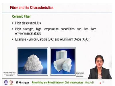
Ceramic fiber is another type of fiber that is used particularly in high temperature where it is required to have high temperature. It has high strength, high elastic modulus and is capable of resisting high temperature and it is free from environmental attack. So, ceramic fibers have the advantage of resisting high temperature.
