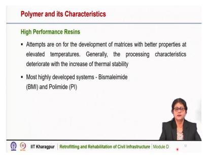
High performance resins, this is actually in research stage and attempts are being made for the development of matrices with metal properties at elevated temperatures. Generally, all these polymers are very susceptible to temperature. So, the research is going on for the development of matrices which can perform better at high temperatures. Generally, the processing characteristics deteriorate with the increase of thermal stability. Most highly developed systems are BMI or Polimide, etcetera.
