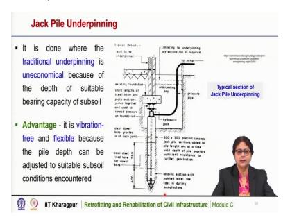
Now jack piling is also used for strengthening purpose. It is done where the traditional underpinning is uneconomical, because of the depth of suitable bearing capacity of subsoil. Sometimes we do not estimate that where is the soil which has sufficient bearing capacity.
