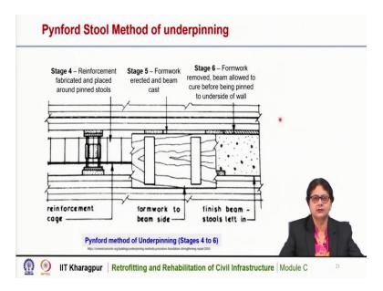
Then in stage four, the reinforcement fabricated and placed around the pinned stool. So, we have a reinforcement cage and that reinforcement is to be placed around this stool. So here we can see that this is the main reinforcement and this reinforcement cage is to be placed within that portion. And in the next stage, a formwork is to be erected.
