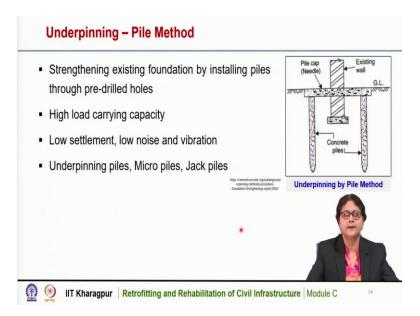
Underpinning by pile method is also quite effective. It is the strengthening technique of an existing foundation by installing piles through pre-drilled holes. The piles have high load carrying capacity and this is an effective method as it causes low settlement, low noise and vibration. So, underpinning by pile method is we can see here in this schematic diagram these are the concrete piles and this is the pile cap and this is the existing wall with its foundation.
