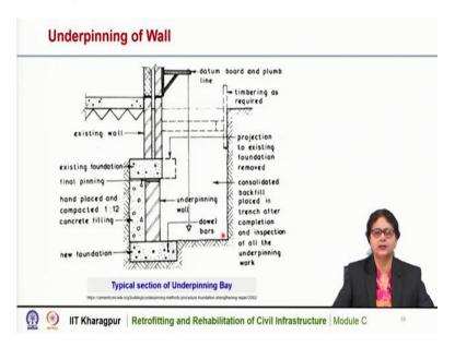
This is a schematic diagram of underpinning of wall. This is a typical section of the under pining bay, we can see here this is the existing wall and this is the existing foundation. Now to support the existing wall, we can cast a new foundation here, but before that the extended portion of the existing foundation need to be removed and before that, pit is to be dug and the existing wall needs to be supported with proper shoring.
