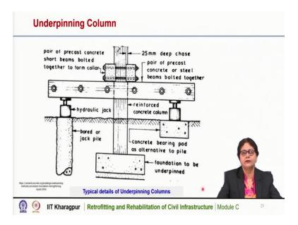
Underpinning column – Sometimes we need to strengthen the existing foundation and the column is reinforced concrete column. So here in this case to strengthen the existing foundation we need to support the reinforced concrete column. Here we can see that this is the RC column, reinforced concrete column and this is the existing foundation.
