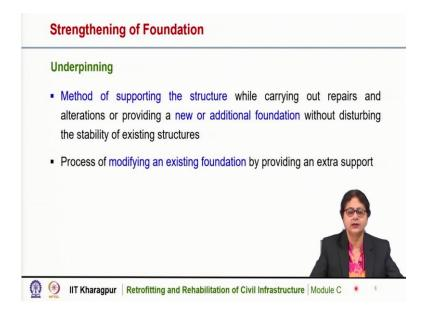
Another technique of strengthening of foundation is underpinning. Underpinning is the method of supporting the structure while carrying out repairs and alterations or providing a new or additional foundation without disturbing the stability of the existing structure. It is the process of modifying an existing foundation by providing an extra support.
