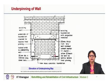
This is the elevation of the underpinning bay. We can see here that this is the existing wall and this is the existing foundation with the projected portion removed. Now this is the underpining wall and this is the new mass concrete foundation within this pit. Now after that the underpinning work this has to be filled up and then it can be ready for taking up the extra load.
