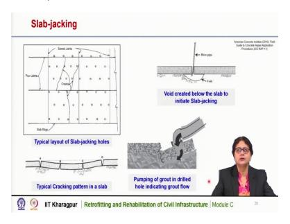
These are the schematic diagrams of slab jacking procedure, you can see here if this is a concrete slab with joints, transverse and longitudinal joints are there and the slab is cracked randomly. As you can see here these are the cracks on the slab. Now for slab jacking purpose, we need to drill a number of holes and these are the holes to be drilled staggered way throughout the slab.
