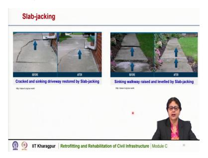
These are some of the pictures of slab jacking, you can see here this is a driveway and the slab is cracked very badly and one portion is settled down, so here this portion is settled down and with slab jacking it is restored, we can see here the portion is restored and they are in one level now. This is also another picture of sinking walkway we can see here; the the slabs are at different levels and by slab jacking procedure the slabs are now in leveled position.
