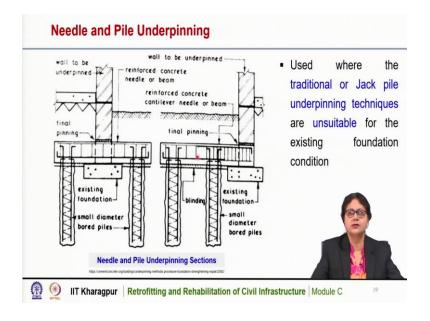
This is needle and pile underpinning. This is used where the traditional or jack piling underpinning method are unsuitable for the existing foundation. So here it is actually the combination of needle beam and the piling method. Here we can see that this is the existing wall and this is the existing foundation. Here we can prepare a needle beam and that is a concrete beam we can prepare and we can also insert piles.
