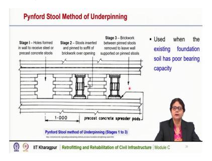
This is another method, Pynford Stool method of underpinning. This is used when the existing foundation soil has poor bearing capacity. So here we can see that this is a schematic diagram of the pynford stool method of underpinning, this is the wall at its elevation we can see the existing wall. So here in this method, several steps need to be followed. In stage one, a hole is formed in the wall to receive the steel or precast concrete stools.
