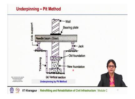
This is a schematic diagram of underpinning by pit method, we can see here this is the wall of an existing structure and this is the existing foundation. In pit method of underpinning, we need to prepare a pit below the existing foundation and it needs to be properly supported by timbering at its sides and now we need to support the wall and we will prepare a new foundation below it.
