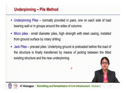
Underpinning piles are normally provided in pairs, one on each side of the load bearing wall or in groups around the side of the column. So, this is underpining piles. Micropiles are small diameter pipes having high strength with steel casing and installed from ground surface by rotary drilling.
