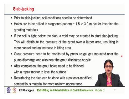
Now there are several steps for slab jacking and we have to follow those steps for this procedure. Prior to slab jacking it is important that soil conditions need to be determined, because we are inserting some grouting materials so we need to know the condition of the existing soil. So, soil conditions need to be determined.
