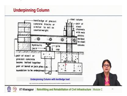
This is also another picture of underpinning column with kentledge load. It is a similar way if we can have only one side accessible then we can use the hydraulic jack here on the bored pile and another one is the pair of steel or precast concrete beams bolted together and this is the kentledge or precast concrete block or similar to act as counterweight.
