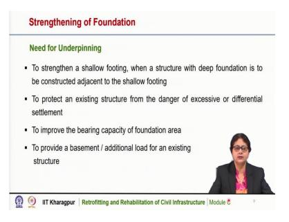
The need for underpining is that to strengthen a shallow footing when a structure with deep foundation is to be constructed adjacent to the shallow footing. For example, a shallow footing is there for an existing structure and adjacent to it a large structure is coming up and for that the foundation may be deeper, so to support or to strengthen the existing shallow for foundation we can do underpinning.
