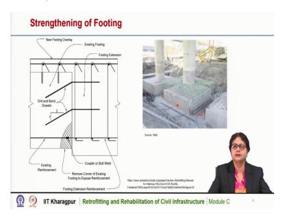
This is the enlarged view of the extended portion of the footing, as you can see this is the existing part and this is the enlarged part. We need to have reinforcement for that and these are the dowel bars which is to be inserted into the existing member and to the new member for proper anchorage and connection.
