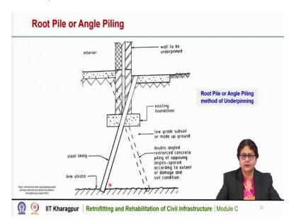
This is another a simple technique of strengthening of foundation. This is root pile or angle piling method. This method involves inserting of the steel linings on both sides of the existing foundation and it is to be done in cross way as we can see here. So, one steel lining is here and the other is here, so in staggered way it can be given.
