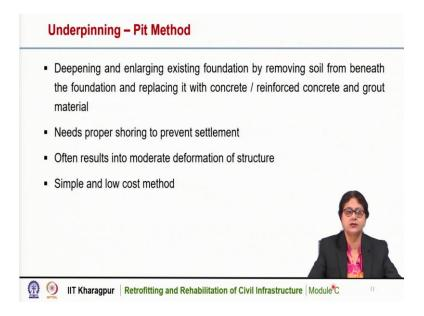
Underpinning using pit method is quite popular and it is used also for strengthening of foundation. Deepening and enlarging an existing foundation by removing soil from beneath the foundation and replacing it with concrete or reinforced concrete and grout material. So here we need to remove the soil beneath the existing foundation and then replace it with a new foundation.
