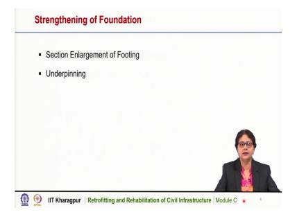
In strengthening of foundation, there are two major techniques, one is section enlargement of footing and the other is underpinning.
