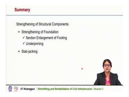
To summarize we have discussed the strengthening of structural components, we have discussed the strengthening of foundation using section enlargement of footing and also underpinning. We have discussed different methods of underpinning using pit method or pile method and we have also discussed slab jacking.
