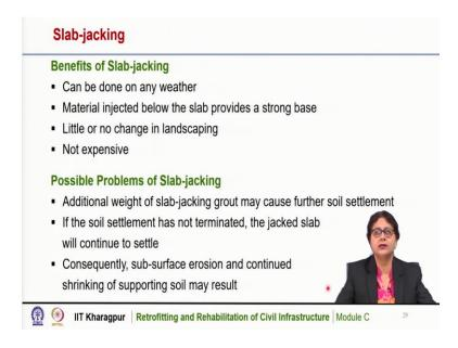
There are several benefits of slab jacking. It can be done on any weather. It does not depend whether it is summer time or winter time, so it can be done on any time. The material injected below the slab, provides a strong base, because we are inserting some grouting material; that is most of the cases it is the cementitious material or some asphalting material and that provides a strong base to the slab.
