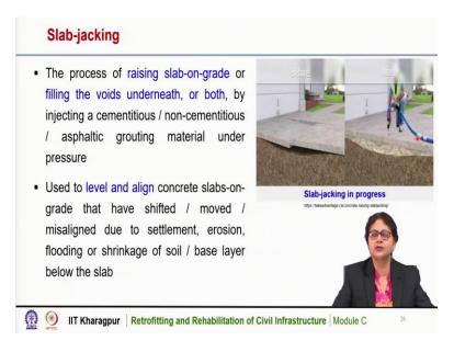
Now, we will discuss slab jacking. Slab jacking is the process of raising slab on grade or filling the voids underneath or both by injecting a cementitious or non-cementitious or asphaltic grouting material under pressure. It is used to level and align concrete slab on grades that have shifted or moved or misaligned due to settlement, erosion or flooding or shrinkage of soil or base layer below the slab.
