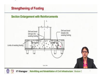
In section enlargement of footing the existing footing is enlarged in its section, as we have seen in case of beams or slabs or columns. The section enlargement is an effective technique for improving the capacity of the member. So, in case of footing also the section enlargement is an effective technique to improve its capacity. So here it is shown schematically that this is the existing footing.
