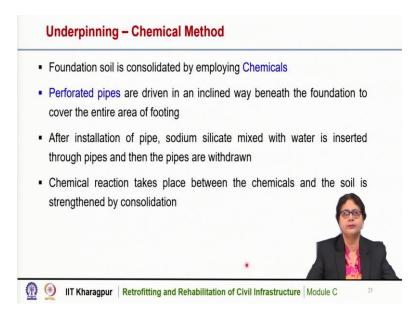
Underpinning can also be done by chemical method. Here the foundation soil is consolidated by employing some chemicals. Perforated pipes are used and the pipes are driven in an inclined way beneath the foundation to cover the entire area of footing. Now after installing the pipe sodium silicate mixed with water is inserted through the pipes and then the pipes are withdrawn.
