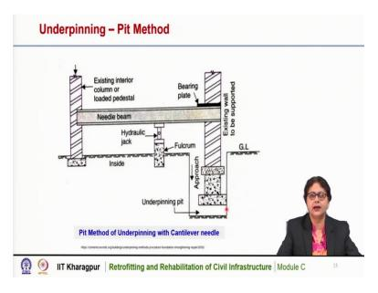
This is also a schematic diagram of underpinning by pit method. Here if the axis is not available on both sides of the existing wall to be supported, then we can do underpining by taking it on the one side only. So here, pit is to be dug, you can see here this is the pit that needs to be prepared below the existing foundation.
