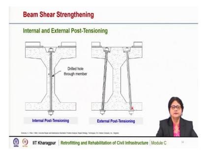
Internal and external post tensioning is done by drilling holes either through the member entirely or through some parts of the member. So, here you can see that this is a concrete girder and a hole is drilled through the member and steel bars or rods or tendons are inserted into it and then it is bolted. So, this way we can do internal post tensioning and then the hole can be filled up by epoxy resin. So, that there is no gap in it.
