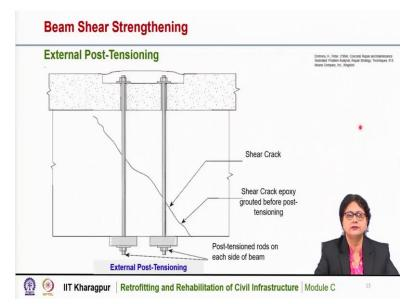
You can see here, in this schematic diagram this is a concrete member and this is a typical shear crack and this is along the length of the member these are typical shear cracks present. So, in that case, we can also do external post tensioning by drilling some part of it and by taking you can see here this part has been considered near the shear crack region and through this part, a hole is drilled and then steel bar, post tension rod is inserted and then it is fixed here.
