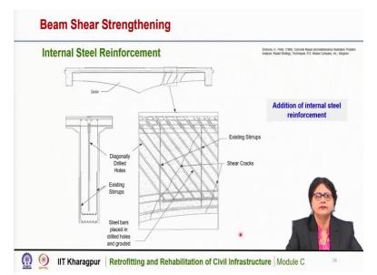
Here you can see that this is a schematic diagram of a girder and there are a number of shear cracks. So, if a more number of shear cracks are there, another technique can also be used using internal steel reinforcement insertion. So, here is what we can do these are the typical shear cracks and perpendicular to these shear cracks, we can drill a number of holes as you can see here, these are the holes to be drilled which are perpendicular to the shear cracks.
