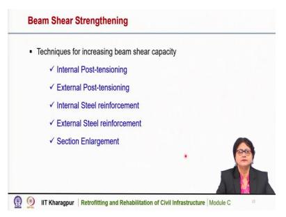
For existing beams, it is sometimes required to improve its shear capacity, there are several techniques for increasing the beam shear capacity like internal post tensioning, external post
