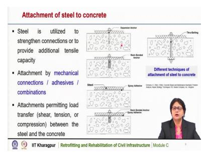
Now, these strengthening techniques we have discussed that can be done either by using new materials or grouting or by stress reduction or post tensioning, etcetera and in many of the cases we need to attach steel plates or steel members to the existing member. So, we have to follow certain, we have to follow certain guidelines for the attachment of steel to the existing structure.
