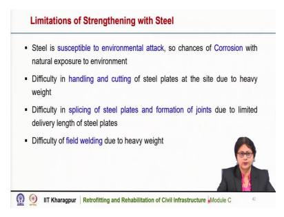
The limitations are that steel is susceptible to environmental attack, and most of the cases the steel straps or tendons or plates are exposed to environment. So, the chances of corrosion are there. And corrosion if it is there then it reduces the effectiveness of strengthening. So, corrosion is a major issue for using steel plates in strengthening of structures.
