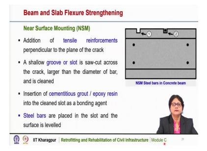
Near surface mounting is another way of improving the flexural capacity of existing members. In this technique, it is the addition of steel reinforcement particular perpendicular to the plane of the crack. So, it is the addition of tensile reinforcement perpendicular to the plane of the crack. A shallow groove or slot is saw-cut across the crack and steel bars are to be inserted into that slot.
