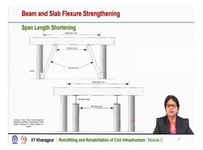
Span length shortening is also another technique, so that the moment on the existing member is reduced. We can use some steel braces, so that the effective span is reduced. And with the reduced span the moment also will be less. So, here is also another technique, you can see here the span length is shortened by placing this type of frame arrangement.
