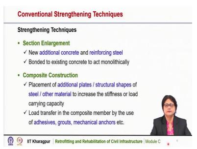
There are several strengthening techniques for existing members. And we will discuss these techniques here. The strengthening could be due to section enlargement, the existing structure is there and we can put additional concrete and reinforcing steel, so that the section of the member now retrofitted is enhanced and the new material should be bonded to the existing concrete, so that they can act monolithically.
