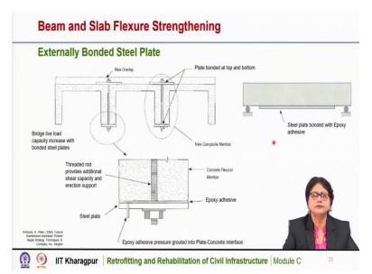
Externally bonded steel plates are effective way of improving the flexural capacity of members. We can see here this is a typical schematic diagram of girder of a bridge, you can see how these are the longitudinal girders and this is the deck slab and if we want to improve its flexural capacity, steel plates can be added at the tension face of the member. Look at this schematic diagram, this is a simply supported beam.
