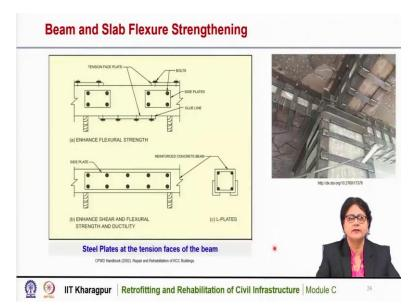
These are also some pictures of attachment of steel plates, at the tension face of the beam, we can also use the plates at the sides you can see here at the bottom or top of the member and also at the sides, we can also use L plates to improve the flexural capacity of the member.
