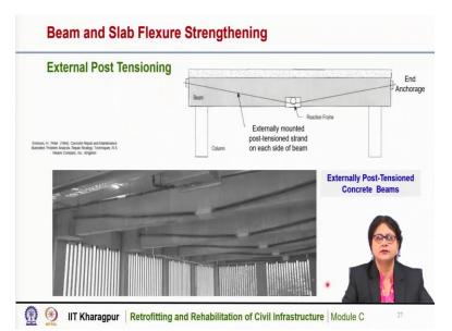
External post tensioning can also be done in this way as you can see with an additional support type of thing with a reaction frame and these are the externally mounted post
