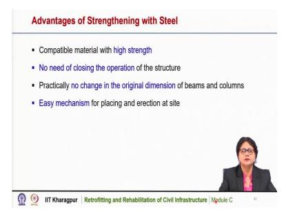
Now, we have discussed that several strengthening techniques using steel plates to improve the flexural capacity, the shear capacity as well as the axial capacity of beams, slabs and column members. So, steel is an effective and useful material for strengthening of existing concrete structures. And it has several advantages and that is why steel is used widely for strengthening and retrofitting of existing members.
