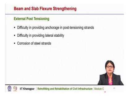
External post tensioning is quite effective and is used widely for improving the strength of existing members. However, it has some limitations; it is difficult sometimes in providing anchorage in the post tensioning strands. Sometimes it is also difficult in providing the lateral stability of the strands and since it is exposed to the environment, so corrosion of steel strands is another issue.
