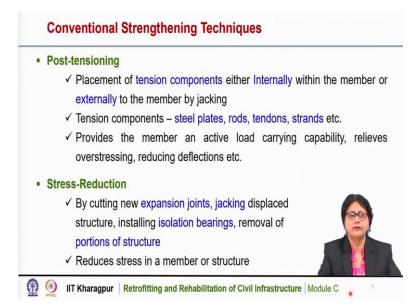
Post tensioning is also another strengthening technique and is widely used. In this technique, it is the placement of the tension components either internally within the member or externally to the member by jacking and the tension components that are used for this purpose are steel plates, rods or tendons or strands, etcetera.
