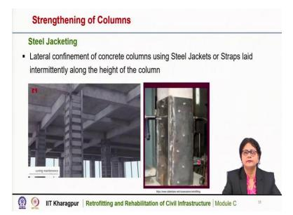
We can also use steel jacketing, concrete jacketing we have seen. A steel jacketing is also an effective means of improving the lateral confinement of concrete columns. The steel jacketing could be continuous steel plate or by steel straps laid intermittently along the height of the column. So, you can see here in this pictures that this is an existing concrete column and to improve its tensile capacity a steel plate all around the column is placed.
