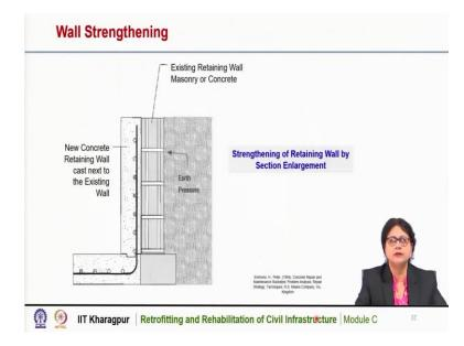
So, we have discussed the flexural strengthening of beams, girders and slabs. Now, the same way, we can improve the capacity of the walls or we can strengthen the walls particularly the retaining walls. You can see here this is a typical schematic diagram of a retaining wall which is supported here and this is the earth on it on this side. And to strengthen the retaining wall a new concrete retaining wall can be cast next to the existing wall with additional reinforcement as you can see.
