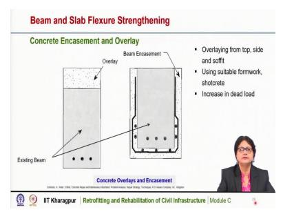
These are pictures of a concrete encasement and overlay. Overlay can be from top of the member or side or soffit or bottom. As you can see, this is an existing beam member with
