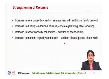
Now, we will discuss strengthening of columns. It is very important to strengthen the columns to increase its actual capacity and this we can do by section enlargement with additional reinforcement. By strengthening columns, we can increase the ductility of the column. By putting additional stirrups or concrete jacketing or steel jacketing. We can increase the shear capacity connection by the addition of shear collar.
