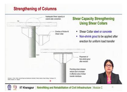
To improve the shear capacity at the of the column slab connection, we can use shear collar. To improve the shear capacity of the column slab connection, we can use shear collars, you can see here, this is a typical shear color, this is made of steel or we can also use concrete for this purpose and then non shrinking grout can be applied after the erection for uniform load transfer.
