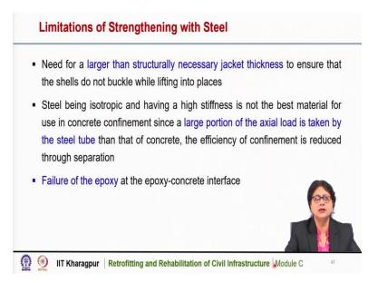
It is also important that we require to have a larger than structurally necessary jacket thickness to ensure that the shells do not buckle while lifting into places. In using steel, sometimes we require a larger than structurally necessary jacket thickness to ensure that the shells do not buckle while lifting into places.
