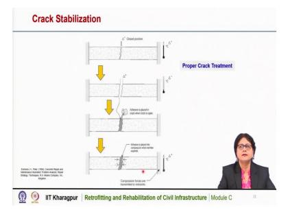
So, when the crack width is maximum, it is desirable to fill up the cracks. In the winter time, when the 2 members may get contracted, so the crack width is much more as you can see here, the crack width is much more as in case of summer time. So, that time we can fill up the crack with epoxy grout or cement grouting.
