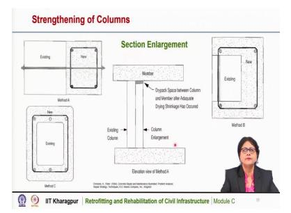
So, to improve the axial capacity of a column member, section enlargement is done. Section enlargement is a common method and it is used also for beams or slabs. And for columns also we can use the section enlargement to improve its axial capacity. So, 3 types of section enlargement can be possible. Here you can see that when the new member is cast just next to the existing member on one side of it.
