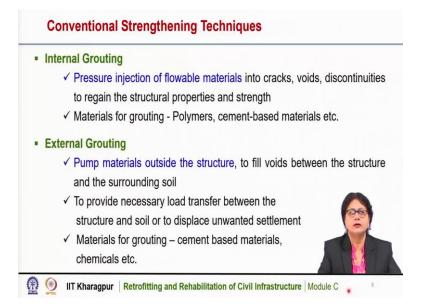
Internal grouting and external grouting are also used for strengthening purposes and they are used for existing structures. In case of internal grouting, it is the pressure injection of loadable materials into the cracks, voids or discontinuities within the member, to regain the structural properties and strength and the materials that are used for internal grouting are polymers or cement based materials or epoxy, etcetera.
